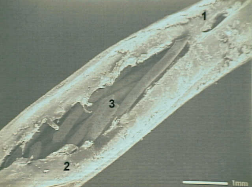
Systems 9 - Exhibit No. 9B - Photo 13. Figure 13g-1. Elemental X-ray microanalysis of damaged Hi-Z shield pigtail lead wire from N93119, sample #29. X-ray microanalysis performed on boxed area (figure 12). Presence of copper & silver on PTFE insulation
