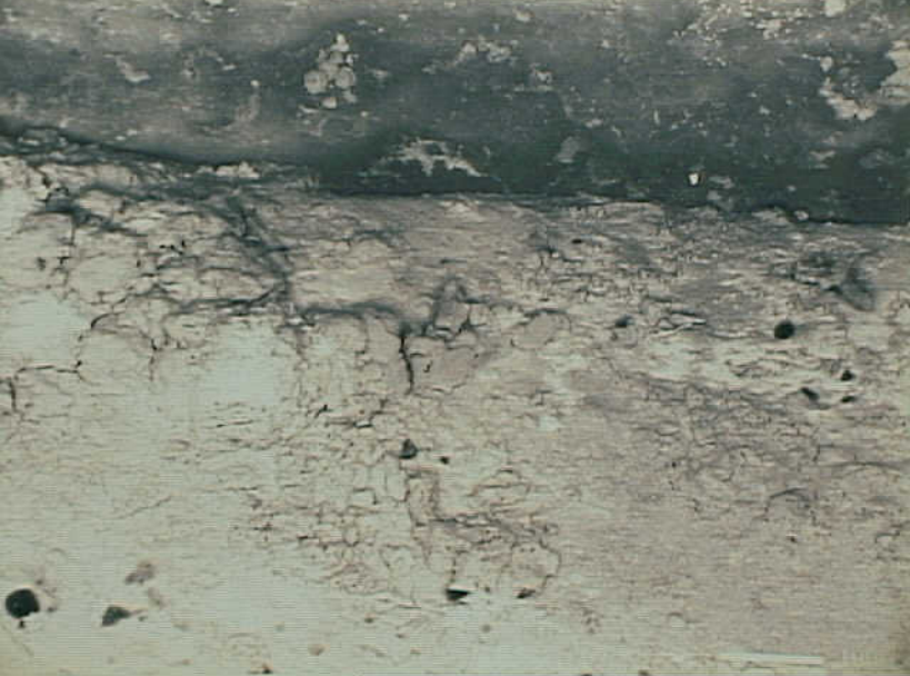
Systems 9 - Exhibit No. 9B - Photo 12. Figure 12b. Base of the relay surrounding the glass to metal seal of N.O. contact A1.
