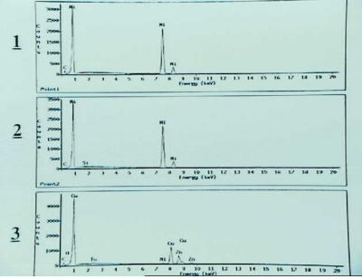
Systems 9 - Exhibit No. 9B - Photo 11b. Figure 11a-2. The areas (1, 2, and 3) of the gouge analyzed using energy dispersive spectroscopy and the resultant
