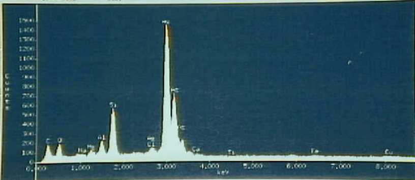
Figure 11. Energy Dispersive Spectrometry (EDS) spectrum of the fibrous material on the moving line contact of the SPR circuit breaker. The silver in both spectra is primarily from the contact material.
