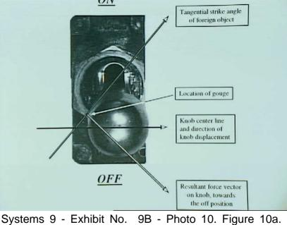
Overall view of scavenge pump switch knob showing the impact gouge (white arrow), the knob center line, the direction of the impact, and the displacement of the knob in the cam groove.
