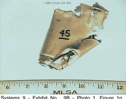
Systems 9 - Exhibit No. 9B - Photo 1. Figure 1g. Sample 45 from N93110 center tank. Typical damage to recovered compensator.
