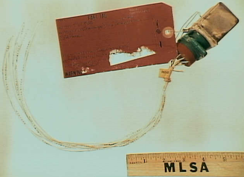
Systems 9 - Exhibit No. 9B - Photo 1. Figure 1b. Scavenger pump relay, as received.
