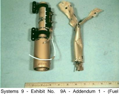
Systems 9 - Exhibit No. 9A - Addendum 1 - (Fuel Probes) Photo 5. Fragment 80 Compensator on right. Similar part on left.
