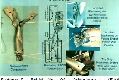
Systems 9 - Exhibit No. 9A - Addendum 1 - (Fuel Probes) Photo 3. Features of Flattened FQIS Compensator (Fragment 80)
