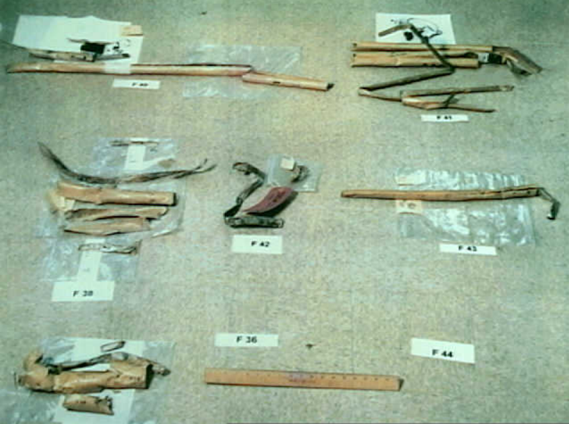
Systems 9 - Exhibit No. 9A - Addendum 1 - (Fuel Probes) Photo 2. CWT fuel probe fragments, as laid out on May 1, 1998. (No negative)
