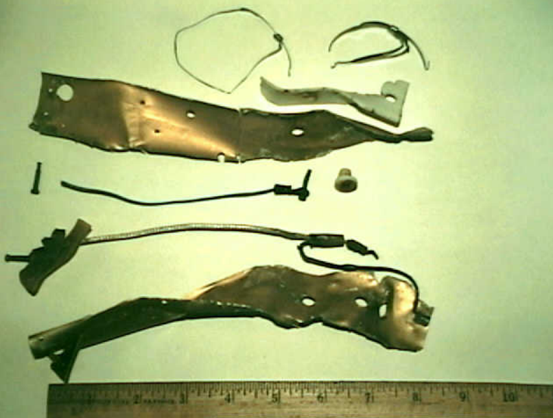
Systems 9 - Exhibit No. 9A - Addendum 1 - (Fuel Probes) Photo 19. Fragment 80 Compensator parts. Ruler is to right of compensator. Loose screw at left is misplaced and is upper HI-Z screw.
