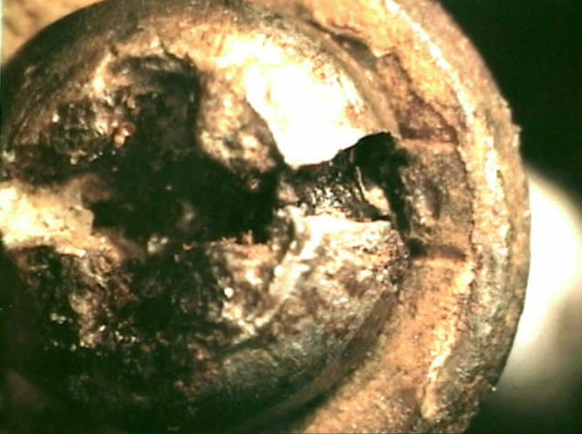
Systems 9 - Exhibit No. 9A - Addendum 1 - (Fuel Probes) Photo 16. Fragment 80 Compensator upper LO-Z screw end ring with alignment of marks.
