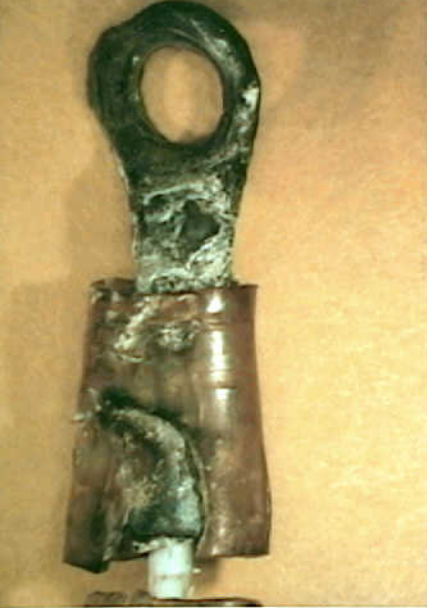
Systems 9 - Exhibit No. 9A - Addendum 1 - (Fuel Probes) Photo 14. Fragment 80 Compensator internal upper HI-Z ring connector front and rear. Darkened plastic visible at bottom.
