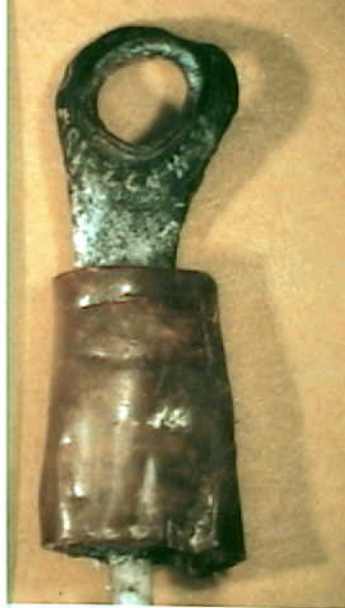
Systems 9 - Exhibit No. 9A - Addendum 1 - (Fuel Probes) Photo 14. Fragment 80 Compensator internal upper HI-Z ring connector front and rear. Darkened plastic visible at bottom.
