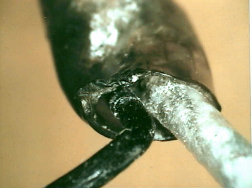
Systems 9 - Exhibit No. 9A - Addendum 1 - (Fuel Probes) Photo 13. Fragment 80 Compensator interior. Bottom of HI-Z splice showing blackened plastic and deformation.
