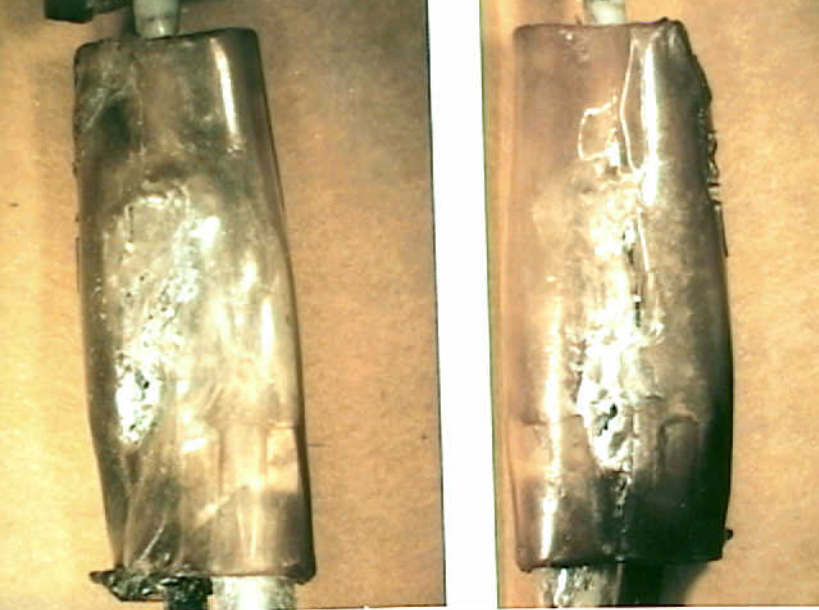
Systems 9 - Exhibit No. 9A - Addendum 1 - (Fuel Probes) Photo 12. Fragment 80 Compensator internal HI-Z splice with blackened features at the bottom. Localized melting visible at bottom of left photo.
