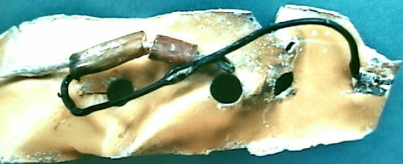
Systems 9 - Exhibit No. 9A - Addendum 1 - (Fuel Probes) Photo 11. Fragment 80 internal HI-Z wire & upper ring connector with splice to shield ground (black wire). Darkened lower features of splice & red insulator are visible.
