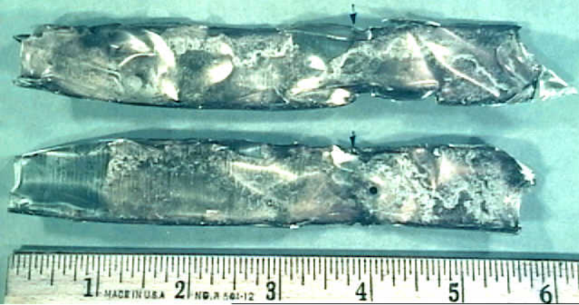
Systems 9 - Exhibit No. 9A - Addendum 1 - (Fuel Probes) Photo 1. CWT aft-most fuel probe fragment (lower tip) interior. The arrows mark change in darkening. (No negative)
