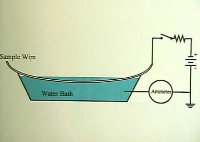
Systems 9 - Electrical Short Circuit/Arcing of Aged Aircraft Wiring - Figure 9. Circuit used for the wet dielectric tests..
