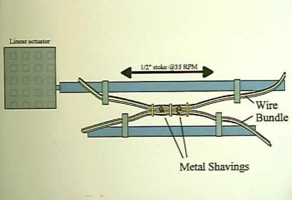
Systems 9 - Electrical Short Circuit/Arcing of Aged Aircraft Wiring - Figure 8. Apparatus used for metal shaving abrasion tests (longitudinal)..
