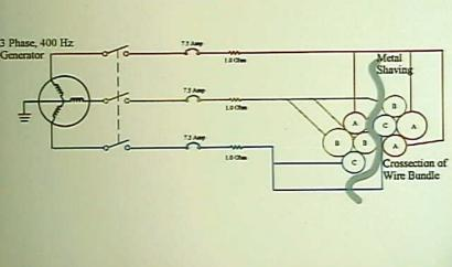
Systems 9 - Electrical Short Circuit/Arcing of Aged Aircraft Wiring - Figure 7. Circuit used for metal shaving abrasion tests (longitudinal)..
