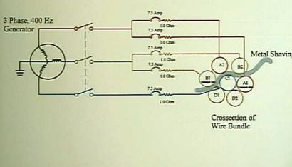
Systems 9 - Electrical Short Circuit/Arcing of Aged Aircraft Wiring - Figure 5. Circuit used in the metal shavings short circuit tests..
