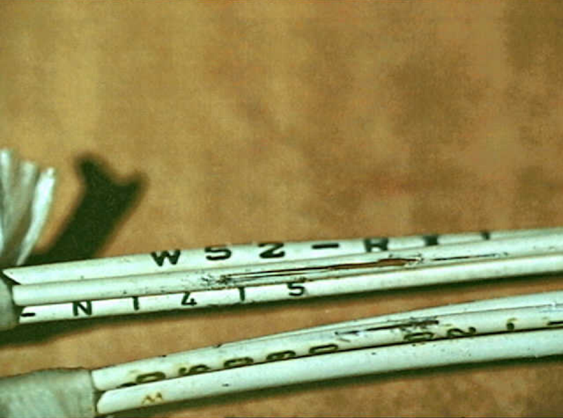
Systems 9 - Electrical Short Circuit/Arcing of Aged Aircraft Wiring - Figure 44. Test 20: Damage done in longitudinal abrasion tests with aluminum 7075
