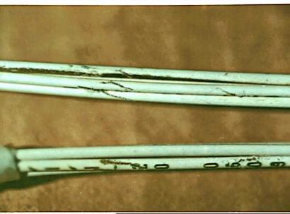
Systems 9 - Electrical Short Circuit/Arcing of Aged Aircraft Wiring - Figure 43. Test 19: Cut damage to the insulation which in some cases reached to the
