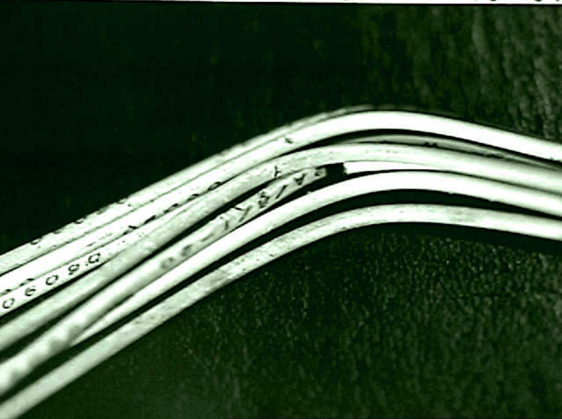
Systems 9 - Electrical Short Circuit/Arcing of Aged Aircraft Wiring - Figure 39. Test 16 A: Damage sample after metal shaving abraders 90 degrees (right angle) test. Note that the broken wire was due to flexing and not the action of the shaving.
