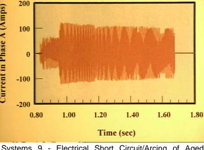
Systems 9 - Electrical Short Circuit/Arcing of Aged Aircraft Wiring - Figure 28. Test 4: Oscillogram of phase A current during a strong arcing event..
