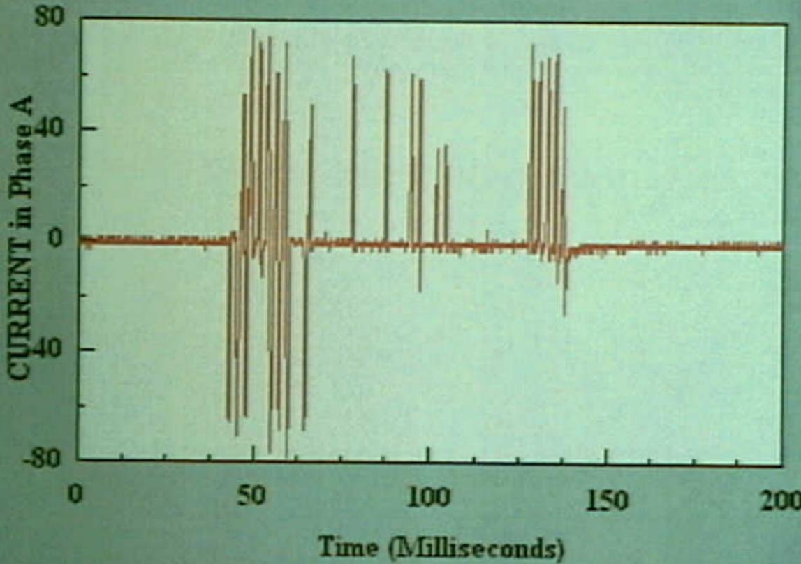
Systems 9 - Electrical Short Circuit/Arcing of Aged Aircraft Wiring - Figure 22. Test 1: Oscilloscope showing intermittent current during a flashing event..
