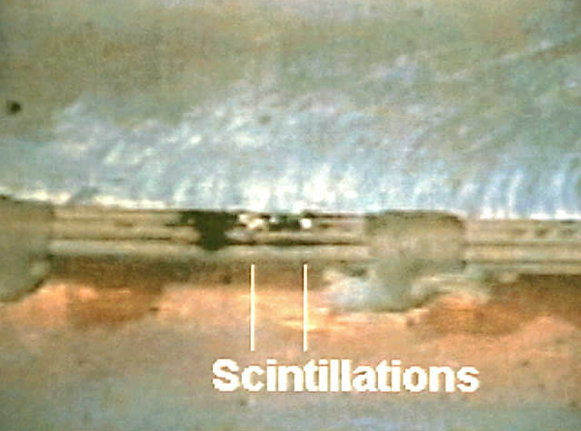
Systems 9 - Electrical Short Circuit/Arcing of Aged Aircraft Wiring - Figure 20. Test 2: Scintillations along the built up char path..
