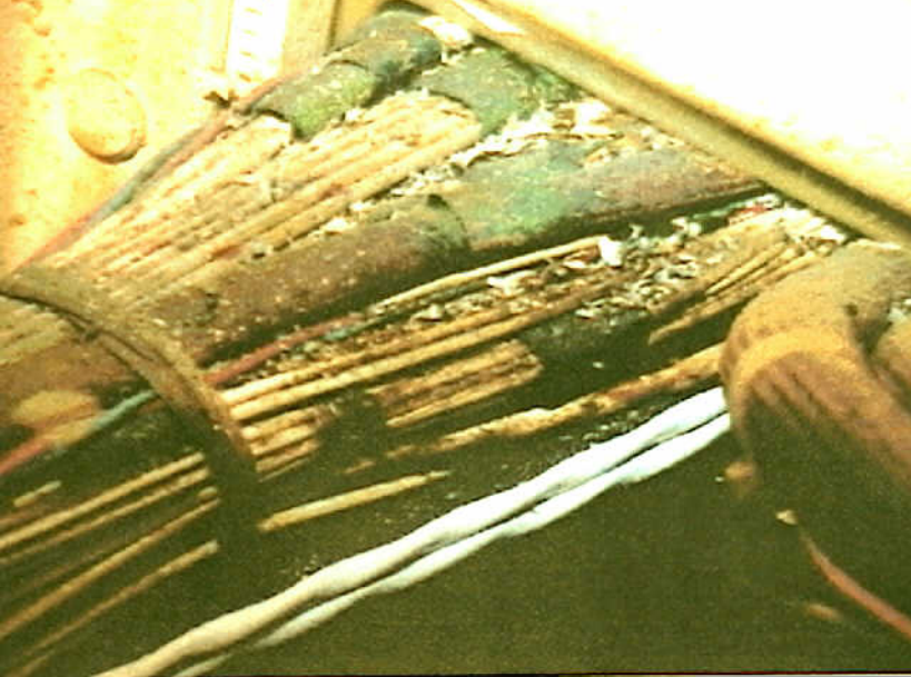
Systems 9 - Electrical Short Circuit/Arcing of Aged Aircraft Wiring - Figure 2. Metal drill shaving on a wire bundle of a commercial aircraft..
