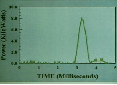
Systems 9 - Electrical Short Circuit/Arcing of Aged Aircraft Wiring - Figure 14. The electrical power dissipated during a flash event..
