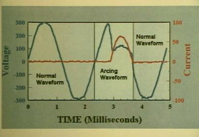
Systems 9 - Electrical Short Circuit/Arcing of Aged Aircraft Wiring - Figure 13. Oscillogram of voltage and current during a flashing event..
