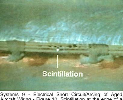
Systems 9 - Electrical Short Circuit/Arcing of Aged Aircraft Wiring - Figure 10. Scintillation at the edge of a pre-damaged crack..
