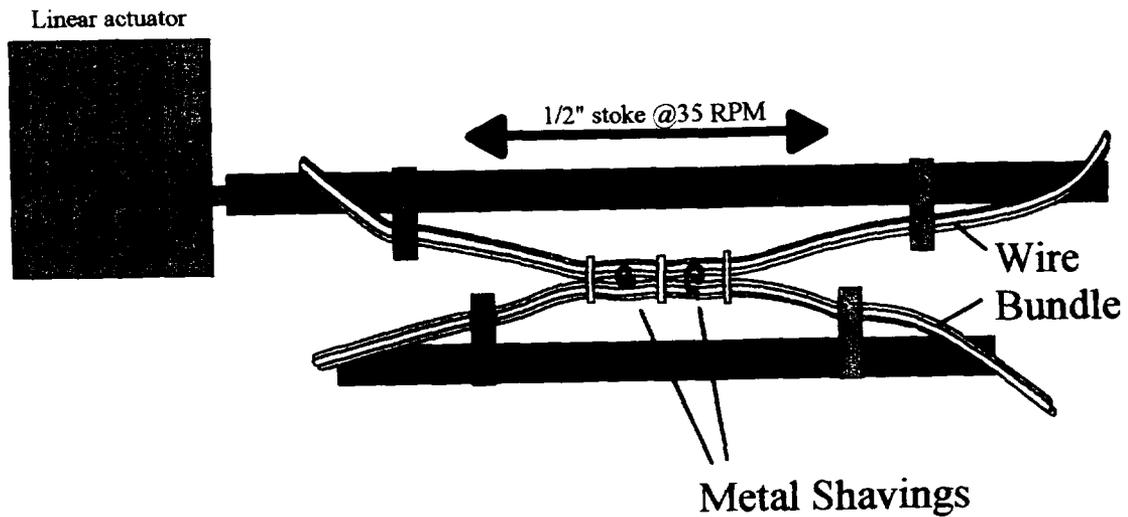
Figure 8. Apparatus used for metal shaving abrasion tests (longitudinal).
