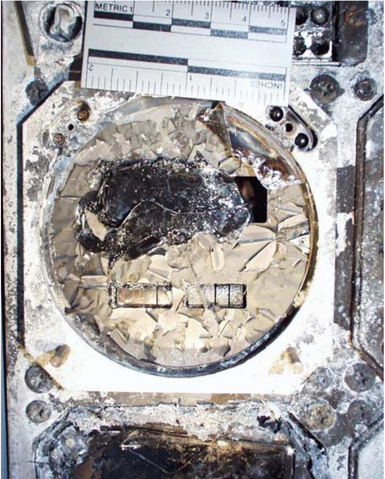
Figure 6-2: Captain's Electric Altimeter
