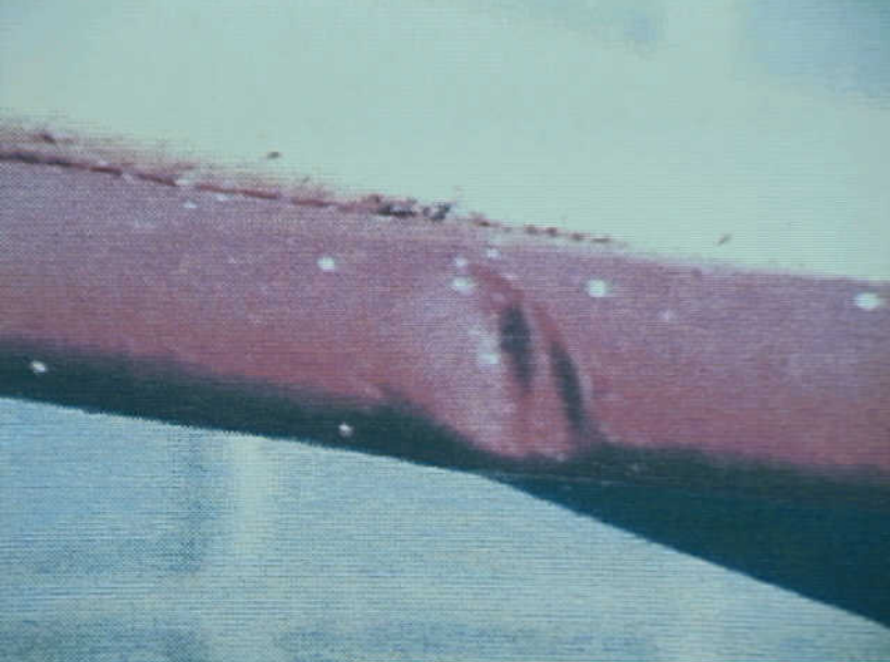
Systems 9 - Aging Aircraft Wire Testing - Photo 13. Gouges in Insulation.
