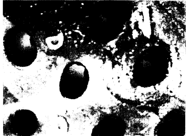
Photo B6: DC10 Sample 6 Connector Grommet deformation and surface crumbling
