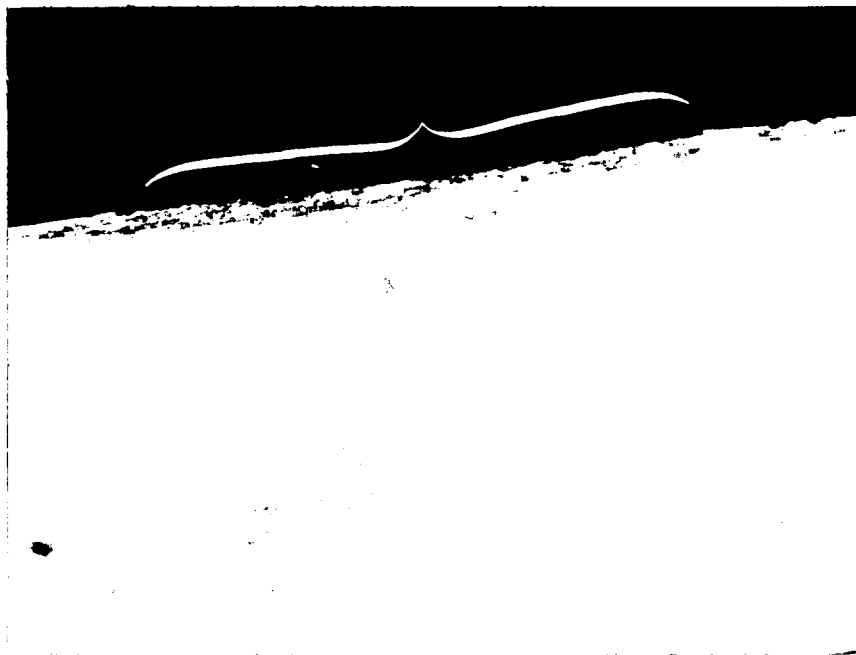
Figure 6. Low magnification micrograph of the cross sectional specimen through the suspect spot showing the minimal corrosion damage along the spot. Keller's etch, 10X.
