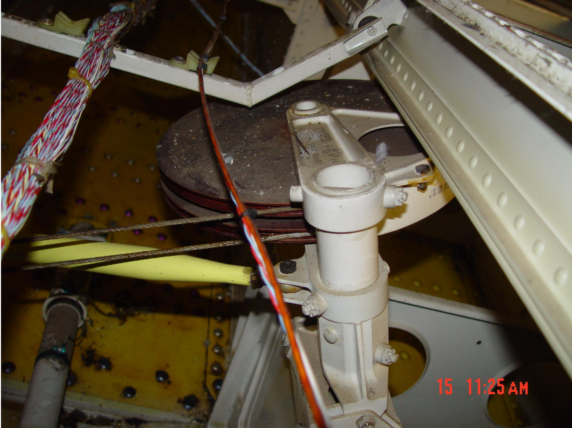
Figure 46. Roll control cable pulley looking forward and down.
