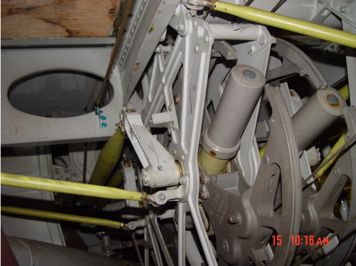
Figure 30. Input rod to roll tension regulator (outboard side).
