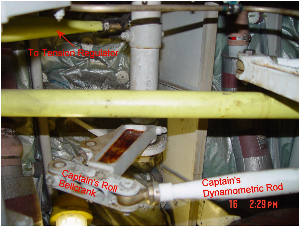
Figure 17. Captain's aft bellcrank and pushrod to tension regulator.
