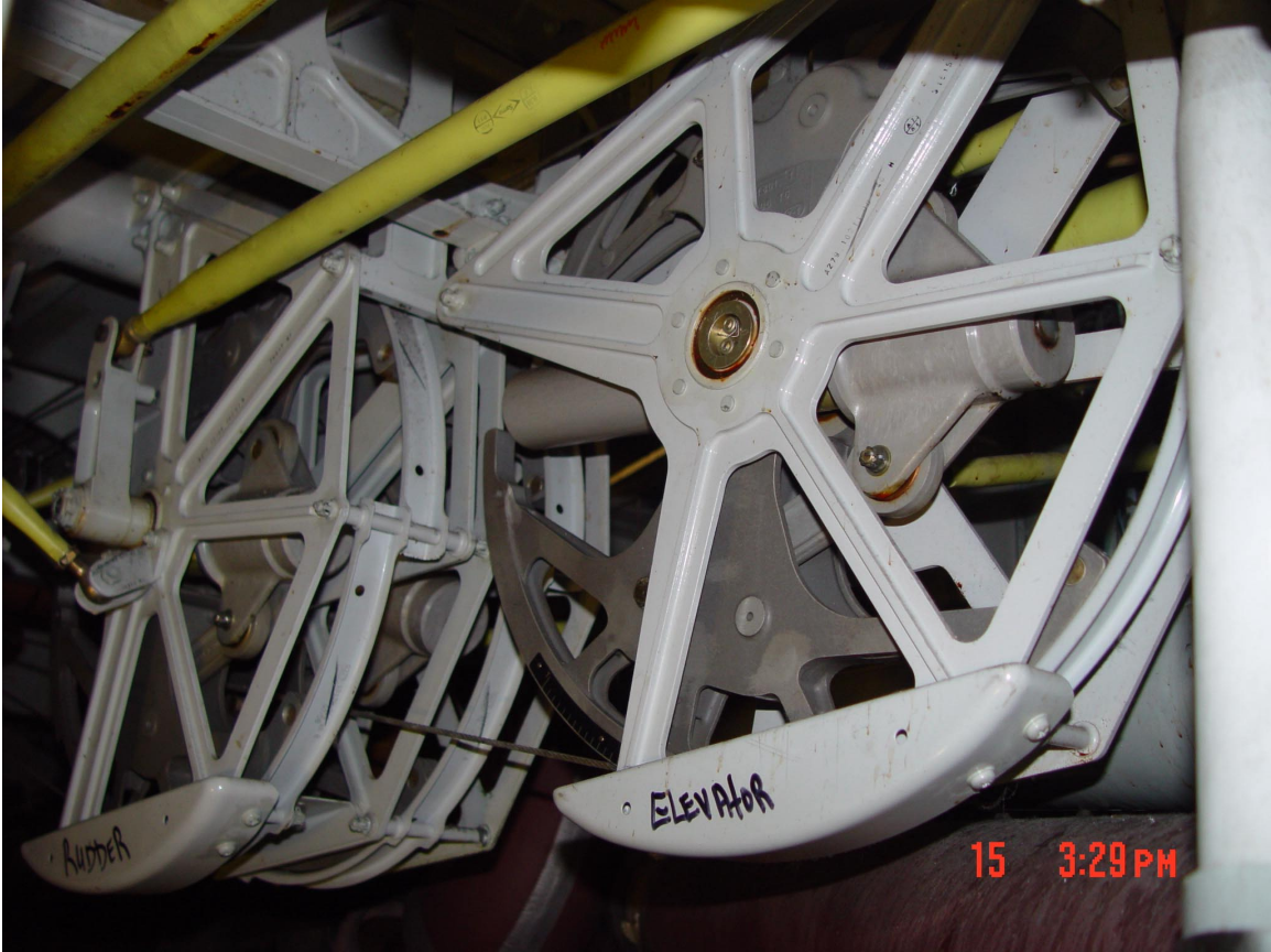
Figure 28. Tension Regulators, left side looking outboard and aft.
