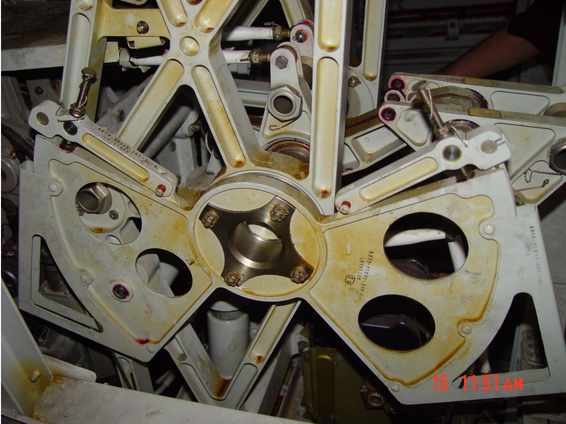
Figure 62. Yaw control cables terminate at quadrant on rudder frame assembly.
