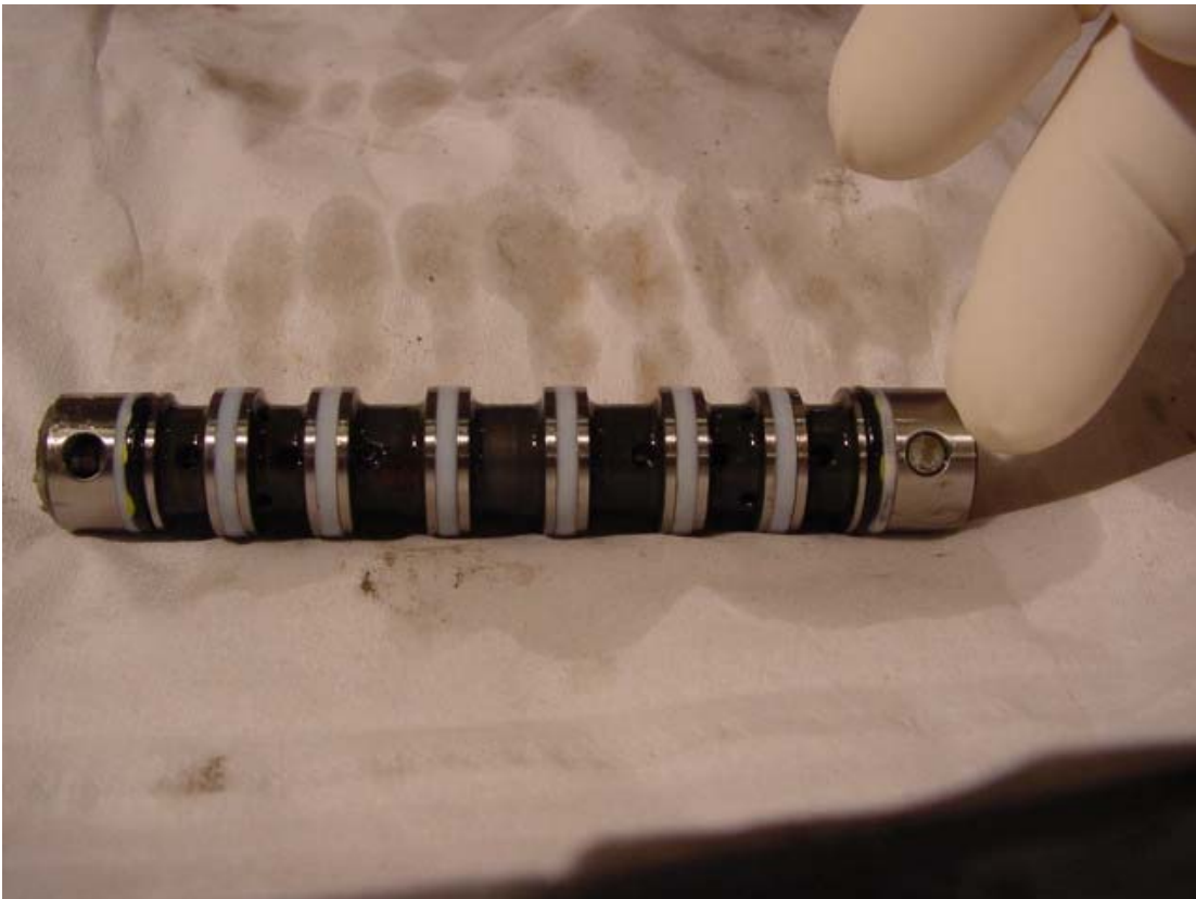
Figure 12. Bypass Valve Cylinder Sleeve.
