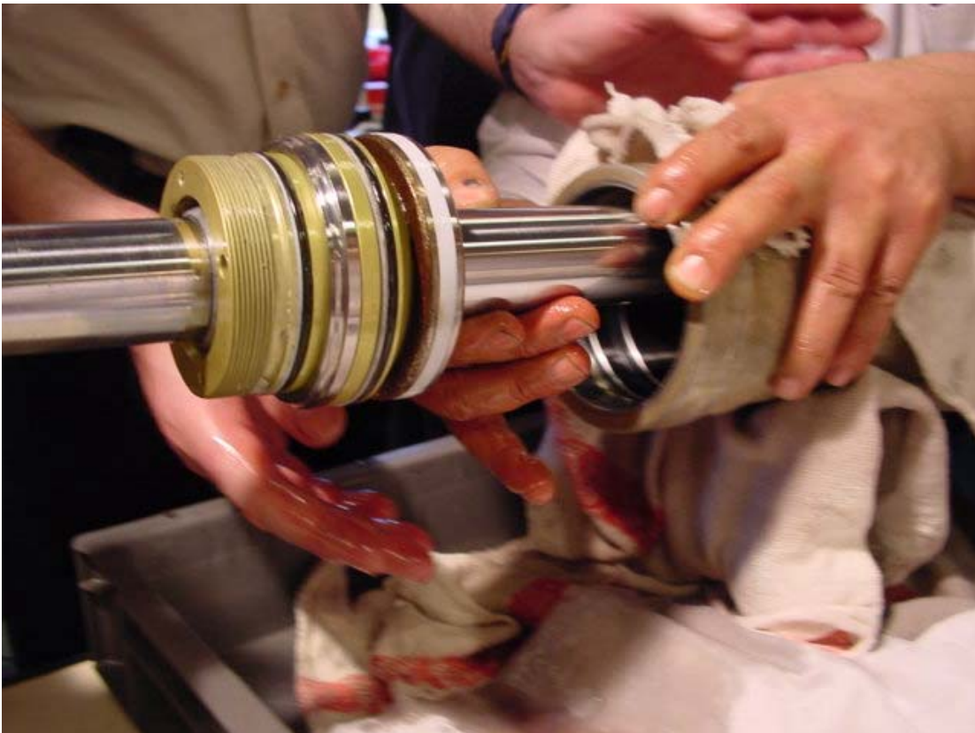
Figure 14. Piston Rod and with Bearing and Seal Assembly.
