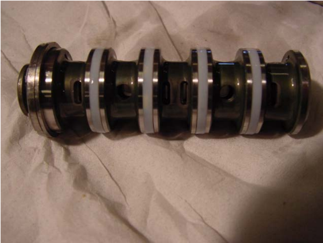
Figure 13. Main Control Valve Cylinder Sleeve.
