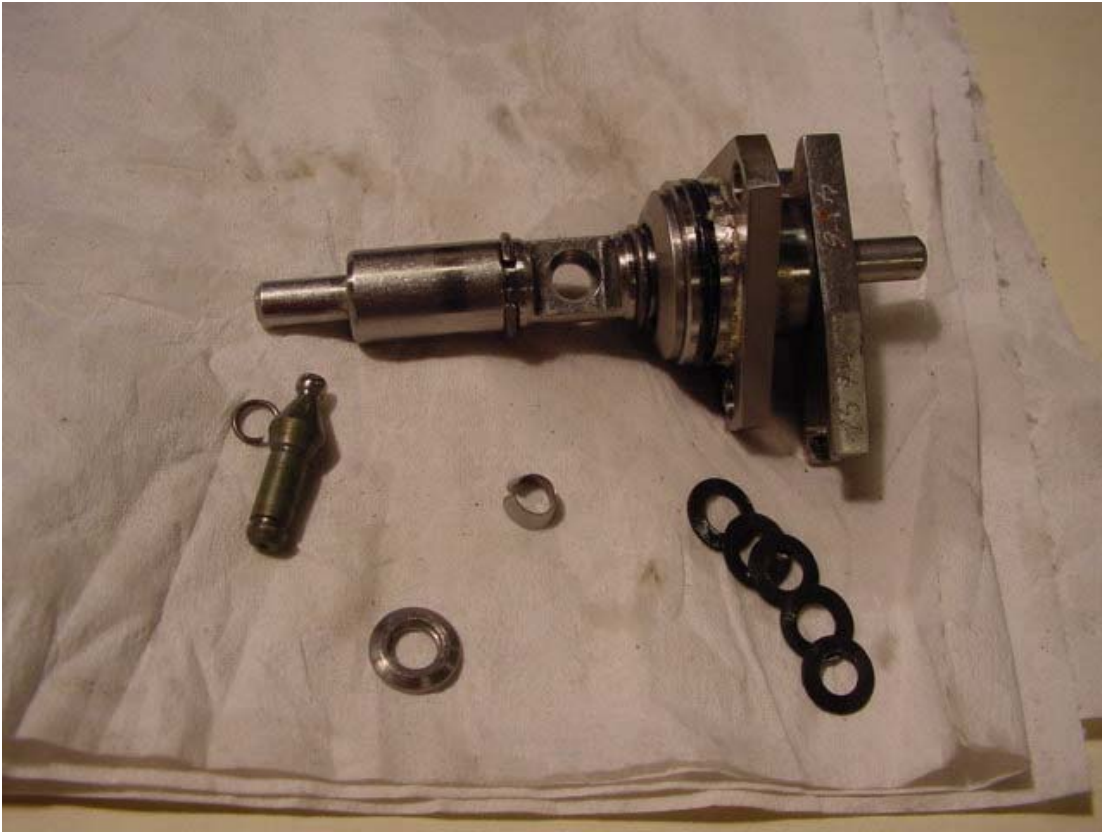
Figure 11. Remote Control Lever with Drive Pin Removed.
