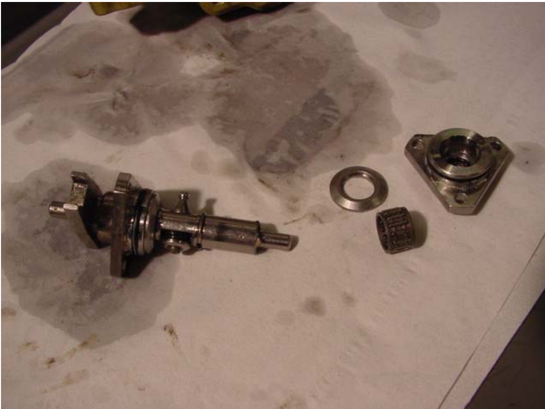
Figure 10. Remote Control Lever and Bearing Assembly
