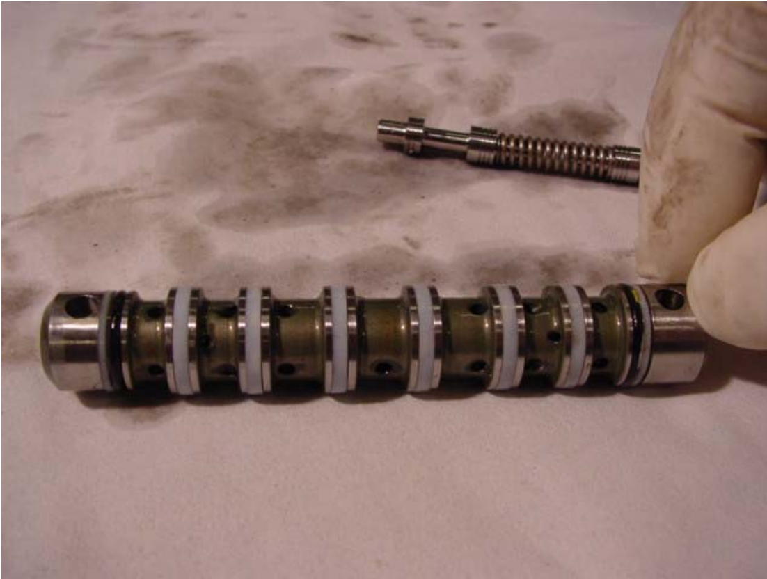
Figure 9. Bypass Valve Cylinder Sleeve.
