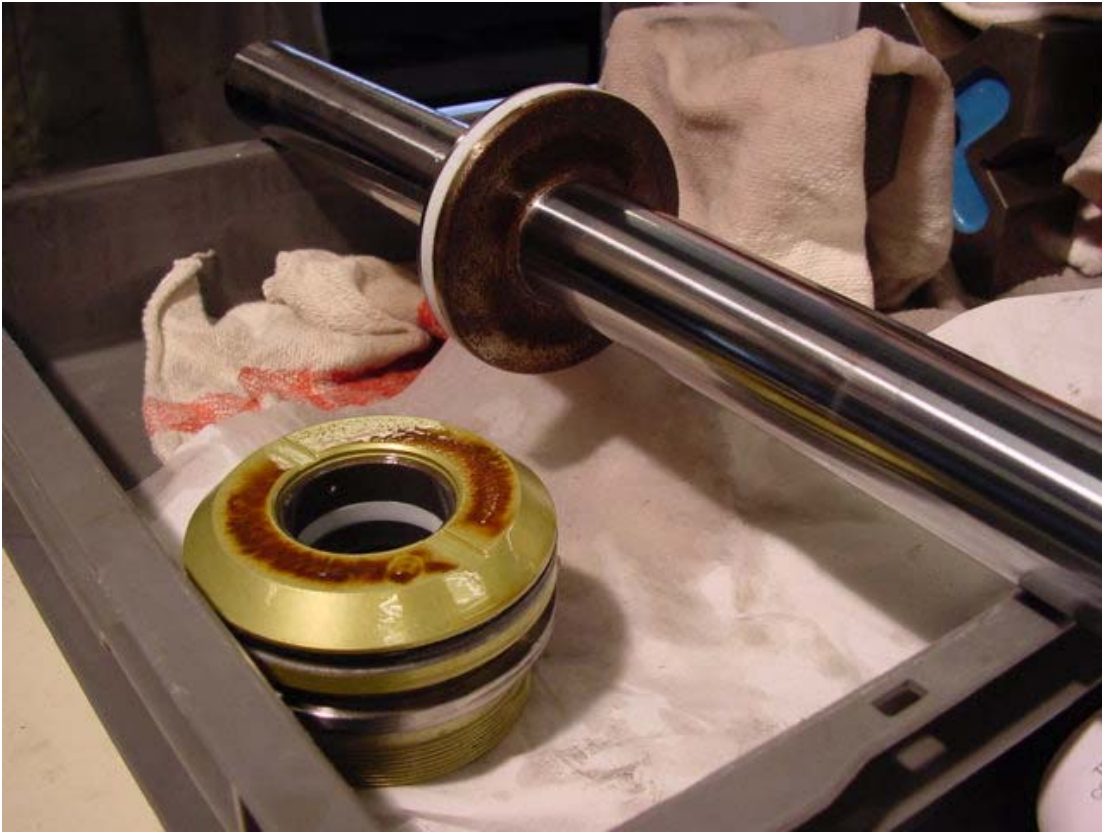
Figure 15. Piston Rod with Bearing and Seal Assembly Removed.
