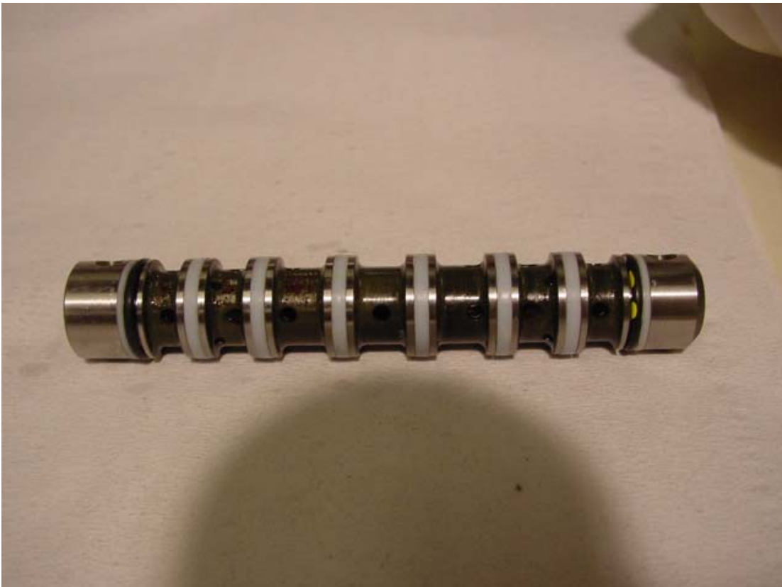
Figure 8. Bypass Valve Sleeve.
