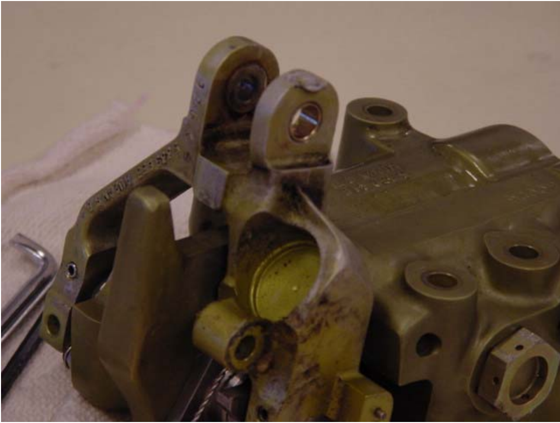
Figure 5. Damage to Input Lever Clevis
