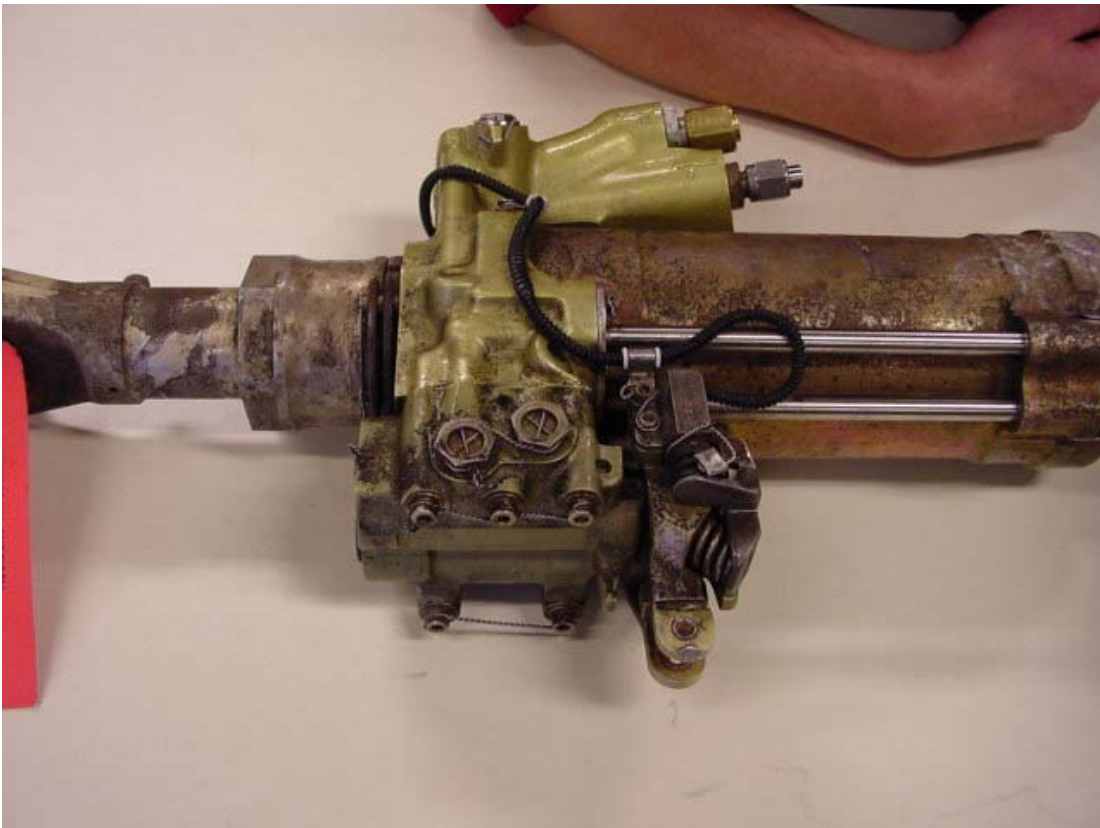
Figure 2. Control Valve Block
