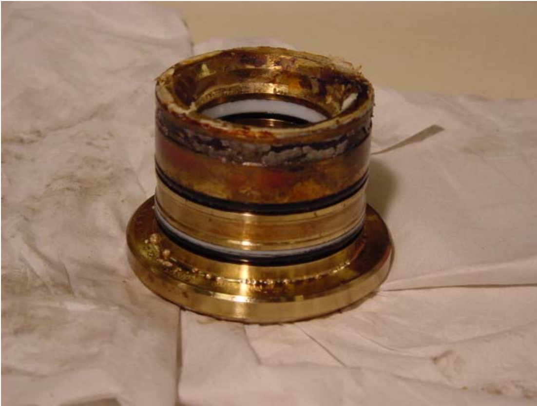
Figure 19. Fixed Rod End Bearing and Seal Assembly.
