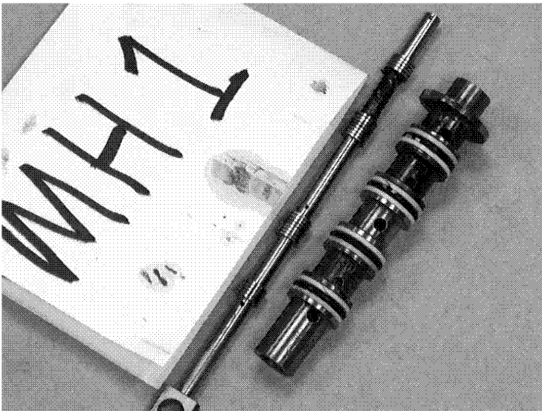
Figure 19, MH #1, Servovalve Slide and Spool
