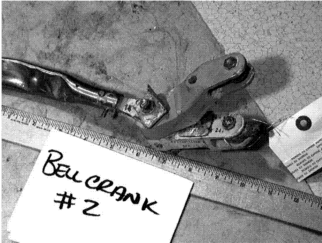
Figure 36, Bellcrank #2, as received in EQA Laboratory
