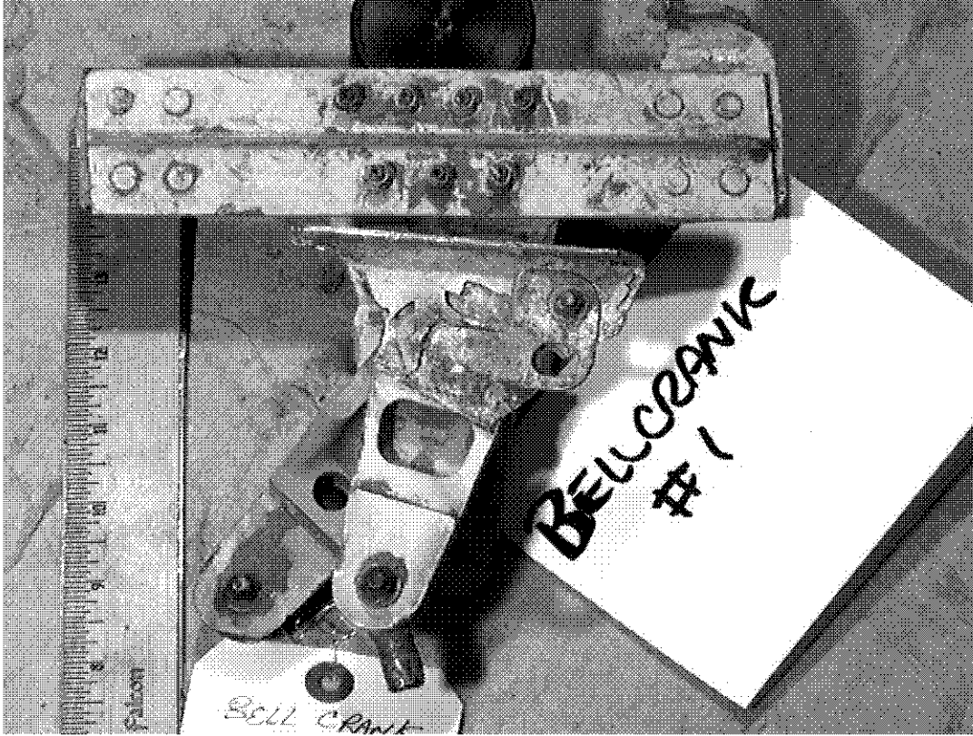
Figure 30, Bellcrank #1, as received in EQA Laboratory
