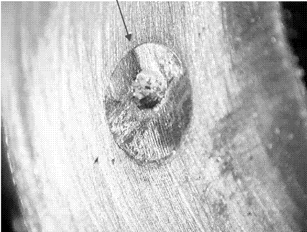
Figure 34, Bellcrank #1, sheared rivet
