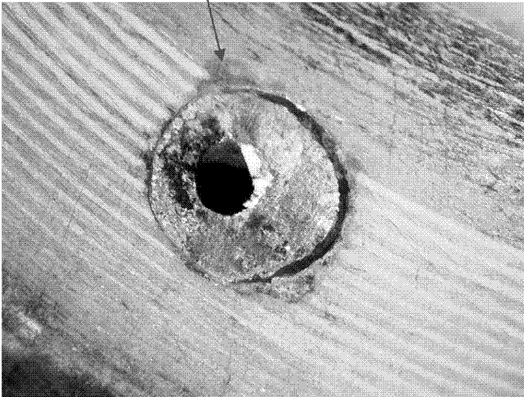
Figure 50, Bellcrank #4, sheared rivet
