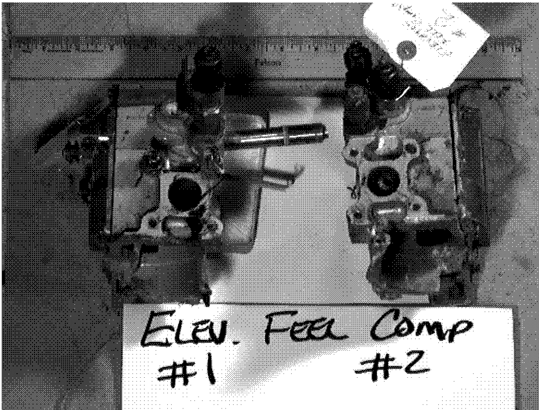
Figure 60, Elevator feel computers #1 and #2, as received in EQA Laboratory
