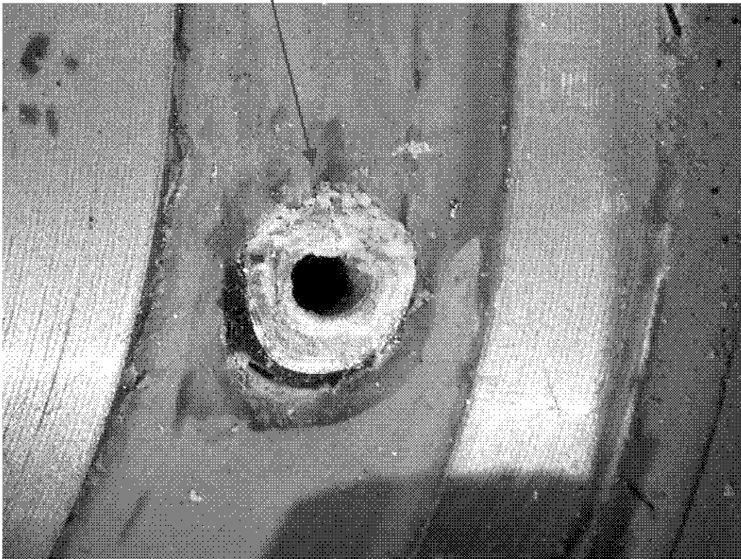
Figure 57, Bellcrank #5, sheared rivet
