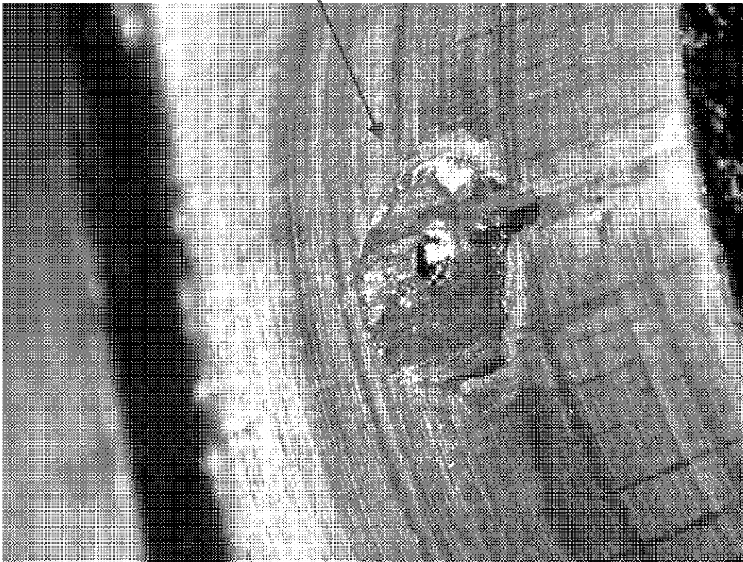
Figure 40, Bellcrank #2, sheared rivet
