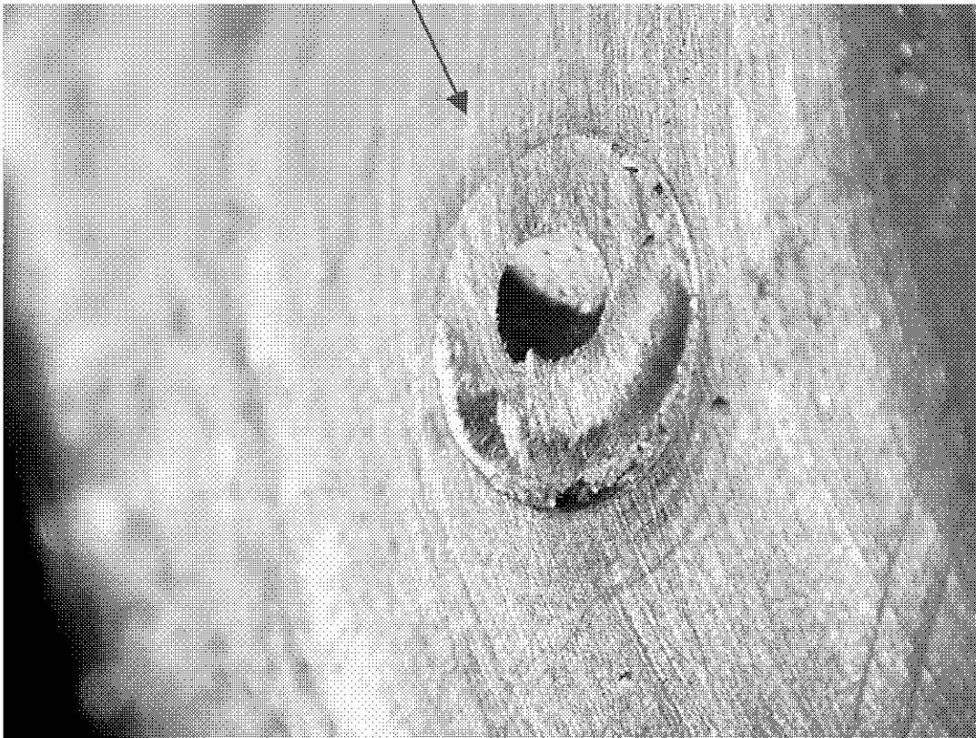
Figure 35 Bellcrank #1, sheared rivet
