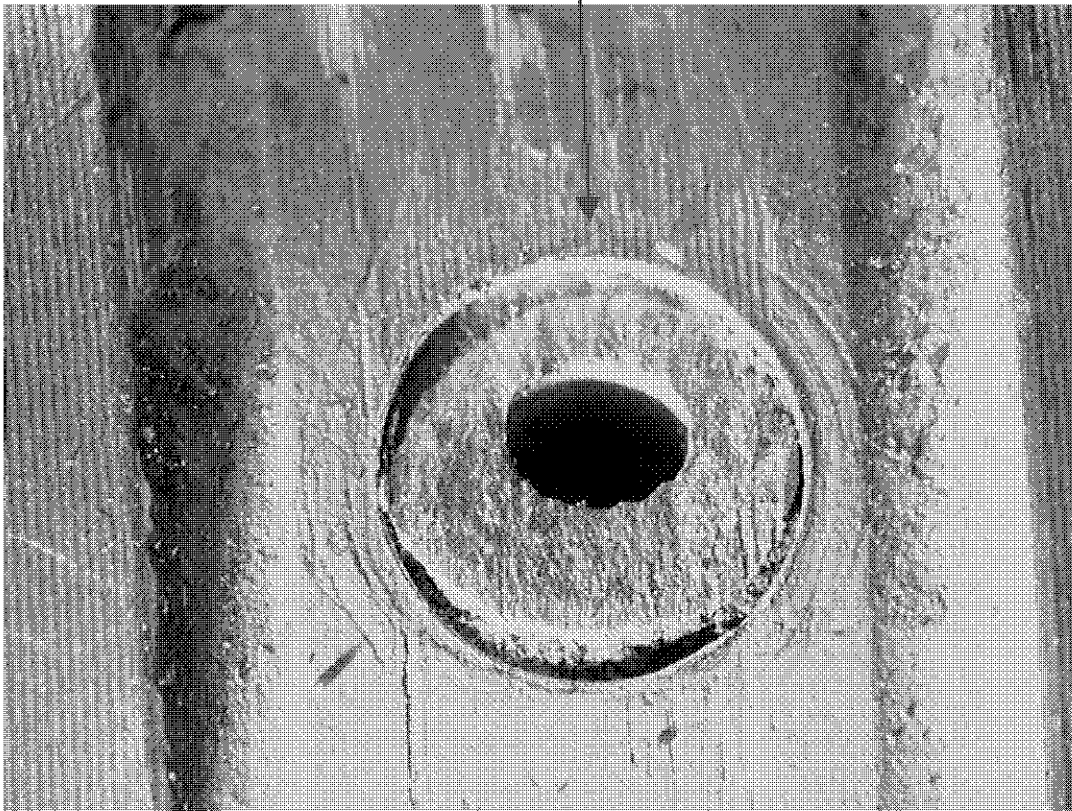
Figure 32, Bellcrank #1, sheared rivet
