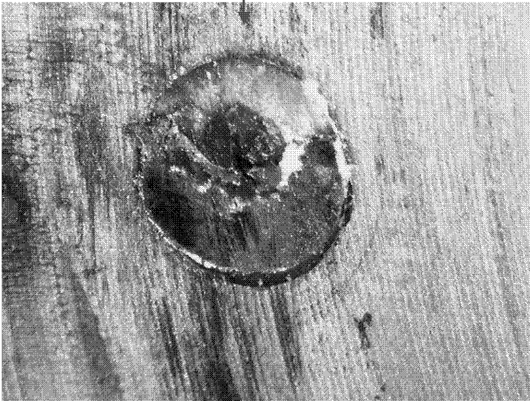
Figure 46, Bellcrank #3, sheared rivet
