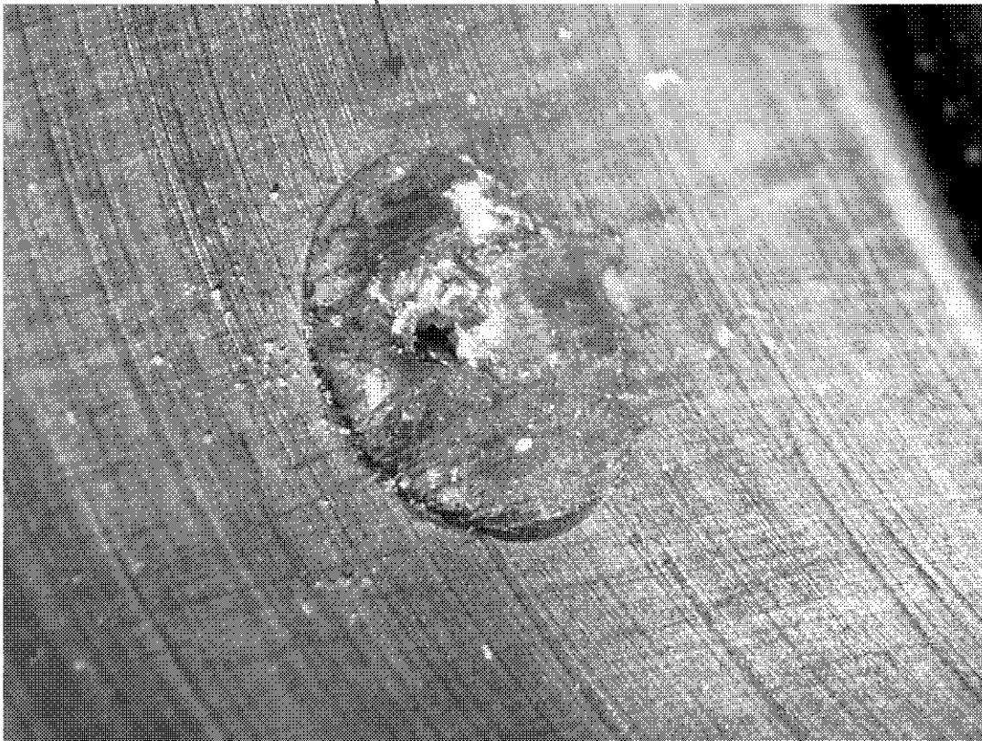
Figure 41, Bellcrank #2, sheared rivet
