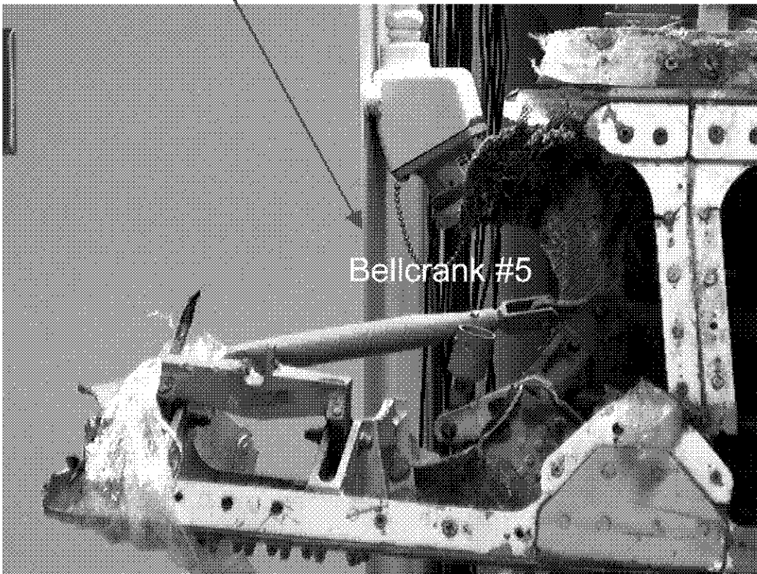
Figure 55, Bellcrank #5, as received in EQA Laboratory
