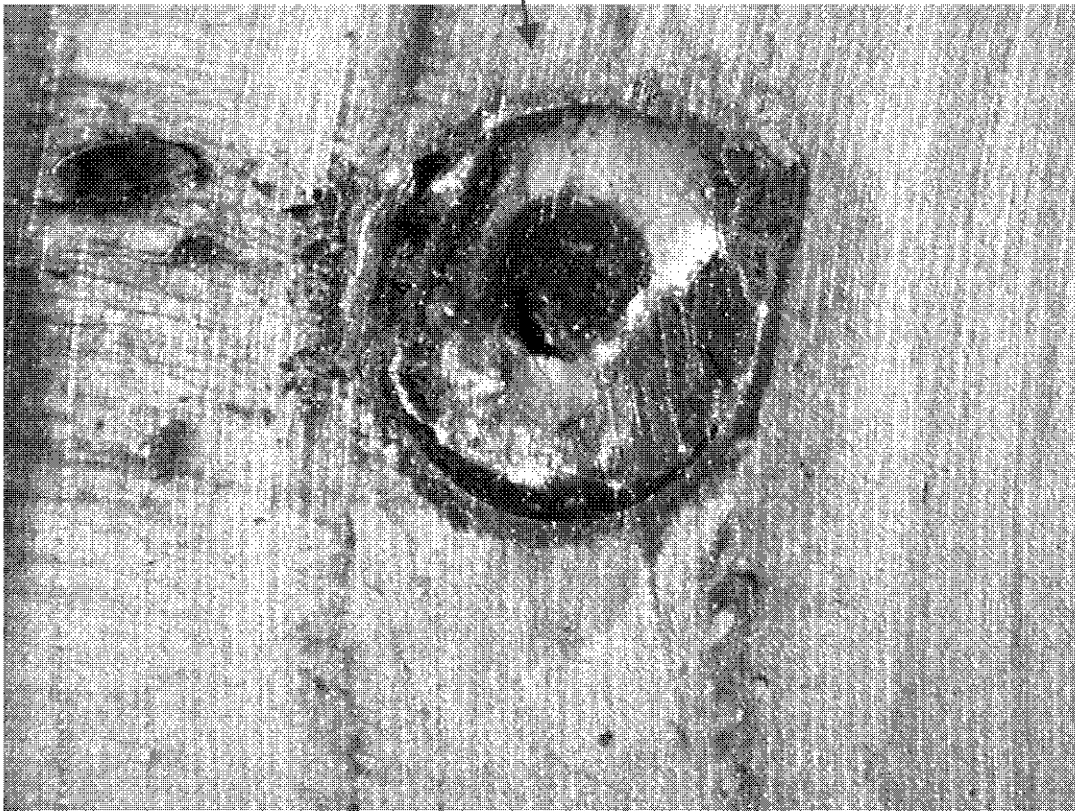
Figure 47, Bellcrank #3, sheared rivet
