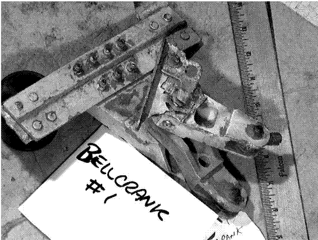
Figure 31, Bellcrank #1, as received in EQA Laboratory
