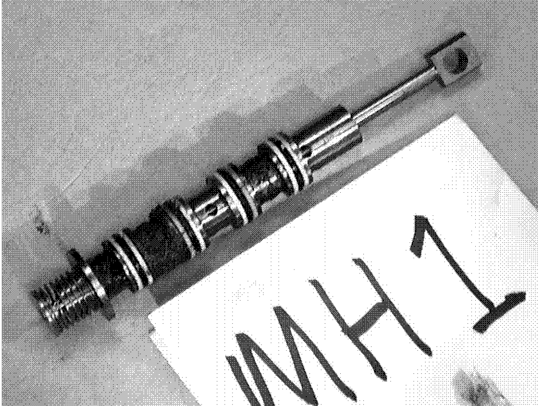
Figure 18, MH #1, Bias Spring, Spring Guide Retaining Cap, Servovalve Slide, & Spool
