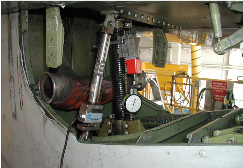
15. Alaska-fabricated strain gauge device imbedded into an Alaska Airlines restraining fixture used during on-wing force output tests.
