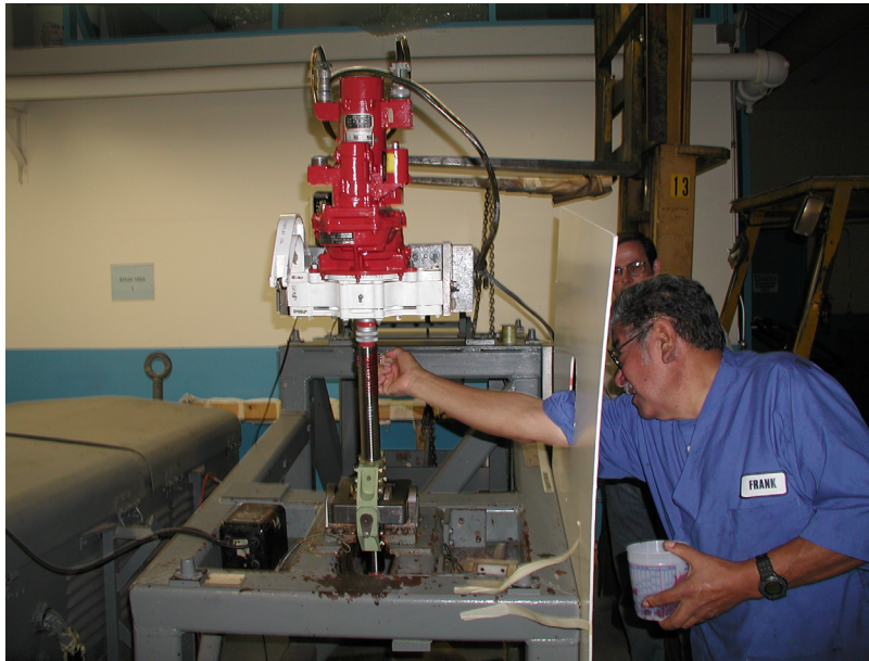
7. Demonstration of grease application onto acme screw only. Grease is being applied with a brush through a mockup of exterior aircraft skin and access panel (Panel is about 10 inches closer to the acme screw on an actual MD-83 aircraft)
