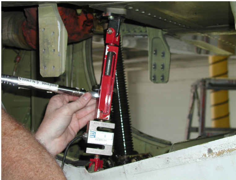
14. Alaska-fabricated strain gauge device imbedded into a Boeing restraining fixture used during on-wing force output tests.
