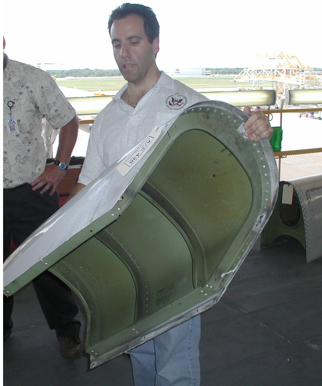
16. NTSB Systems Group Chairman holding an MD-80 “dog house” that fits on top of the vertical stabilizer. The dog house from the accident airplane was missing from the tail assembly and never recovered.
