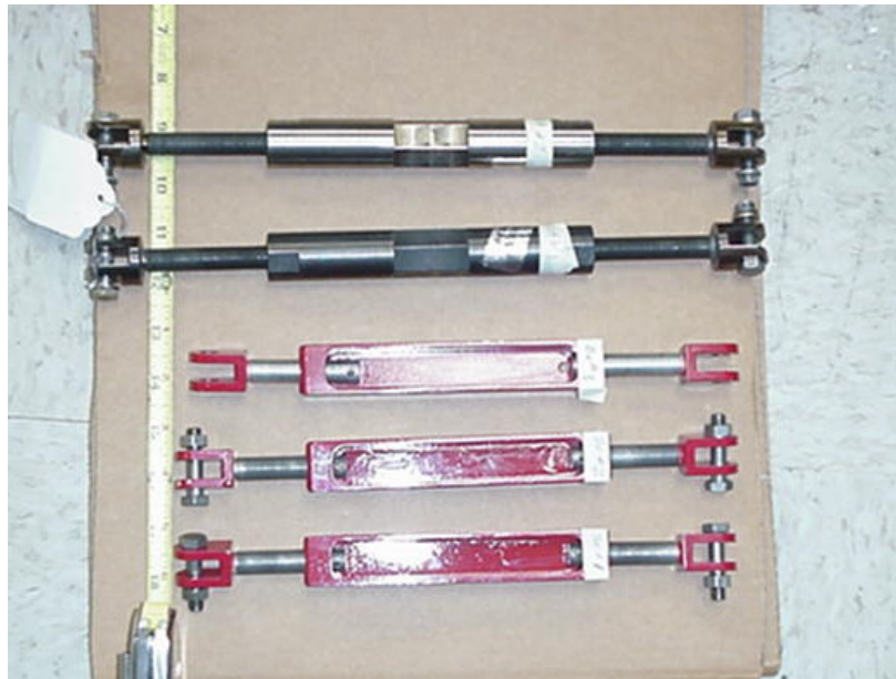
12. View of the 2 Alaska Airlines fabricated restraining fixture tools (top) and the 3 Boeing restraining fixture tools used during the Huntington Beach Laboratory Force Output tests. Note the difference in length, shape, and configuration between the two types of tools.
