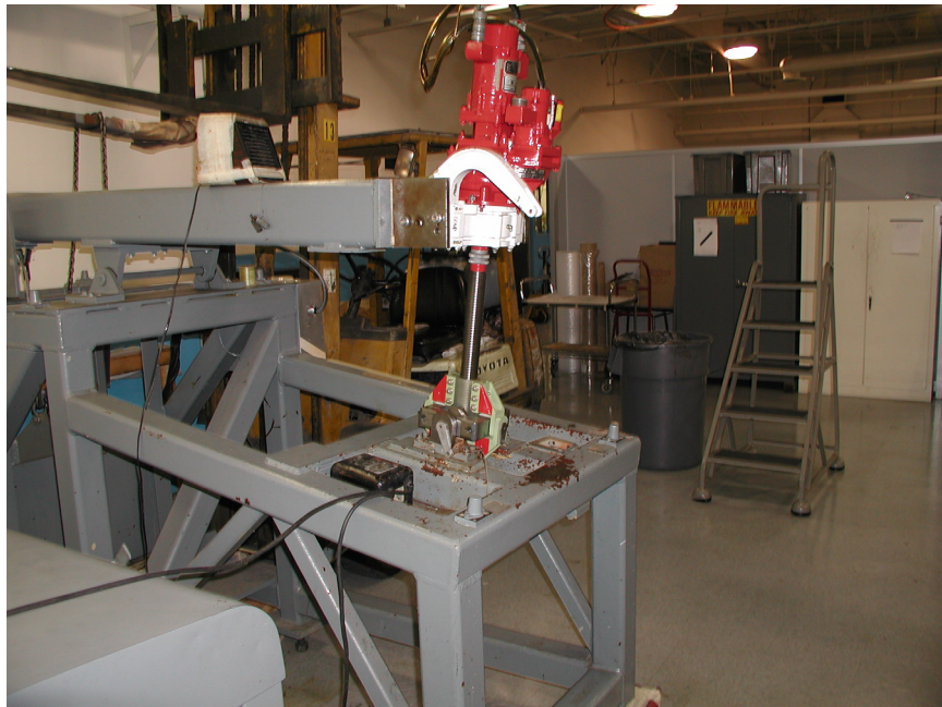
2. Acceptance Test Plan fixture used for acme nut demonstrations at Integrated Aerospace
