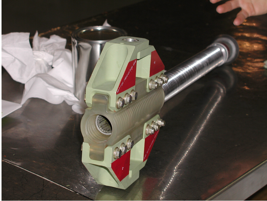
1. Translucent acme nut used in lubrication demonstration at Integrated Aerospace.
