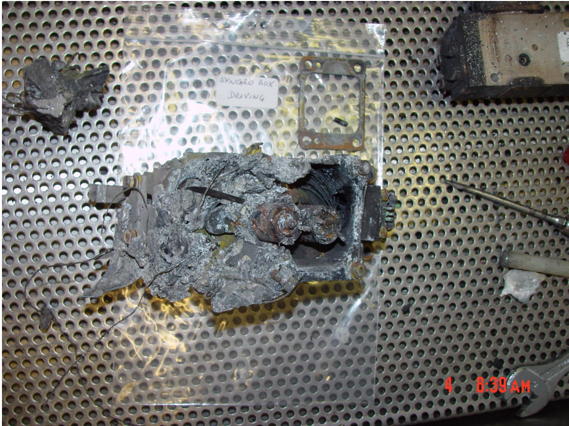
Figure 13. Driving Side Synchro Box Removed.
