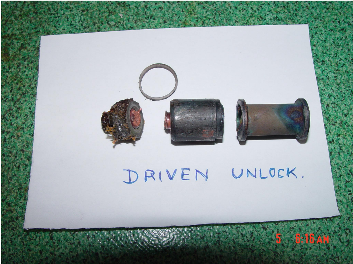
Figure 27. Driven Side Unlock Piston.
