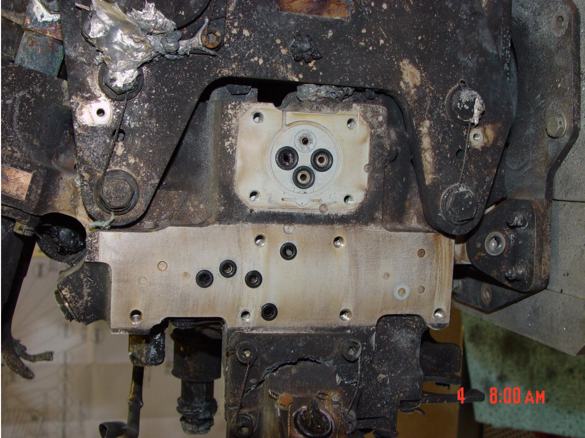
Figure 5. Driven Side of Actuator with Servovalve and Hydraulic Block Removed.
