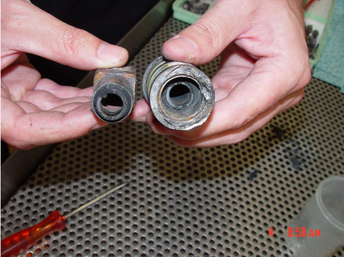
Figure 15. Driving Side Locking Cam Linkage Removed (fractured).
