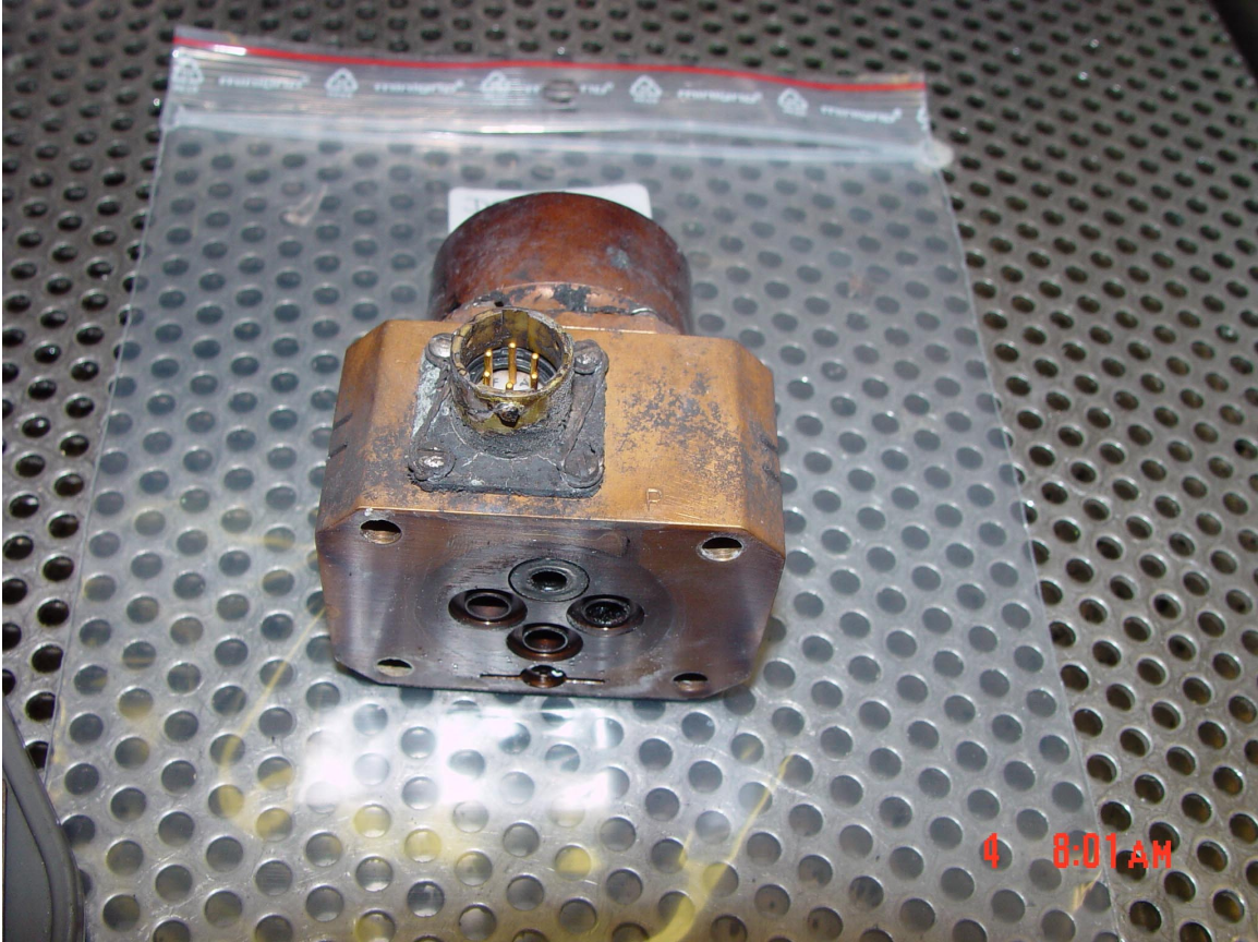
Figure 6. Driven Side Servovalve.
