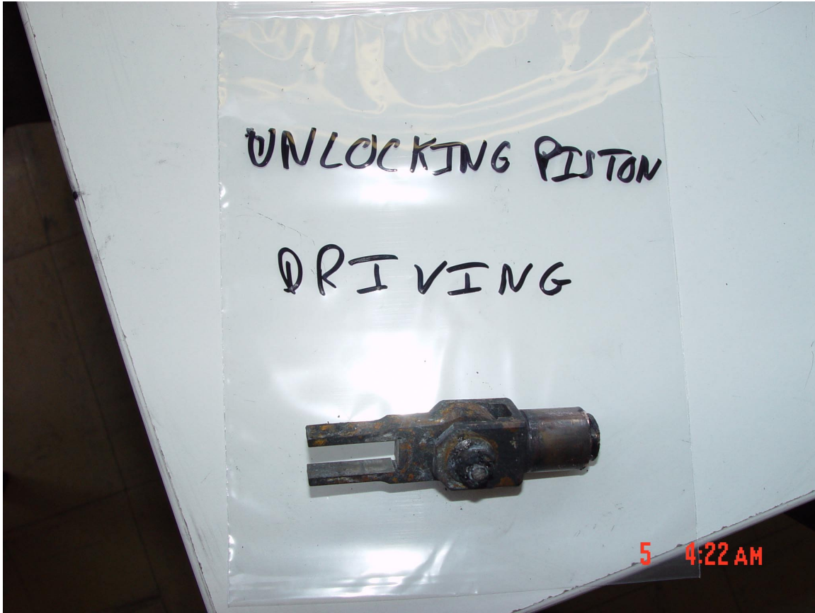
Figure 25. Driving Side Unlocking Piston and Fork (fractured).
