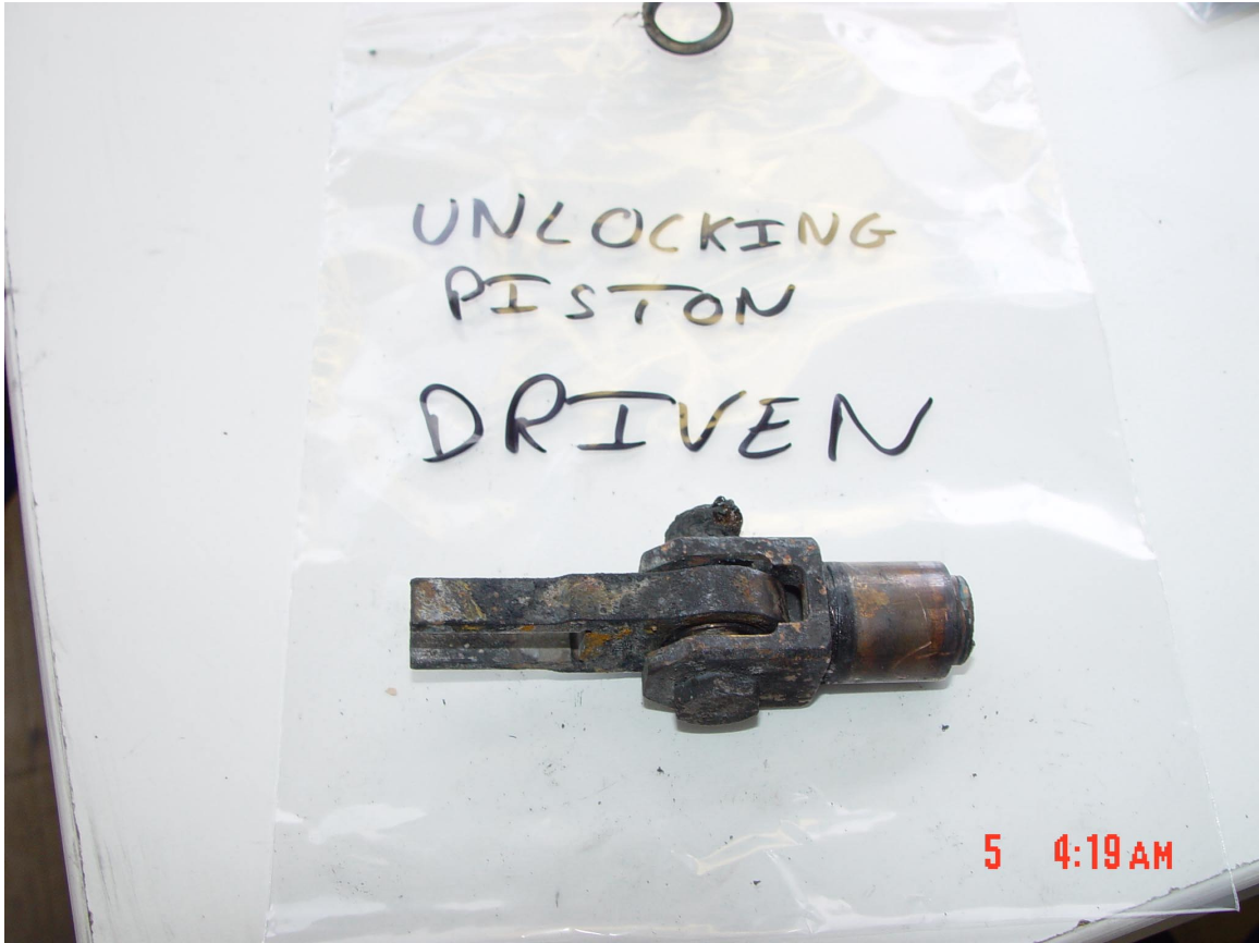
Figure 23. Driven Side Unlocking Piston and Fork (fractured).
