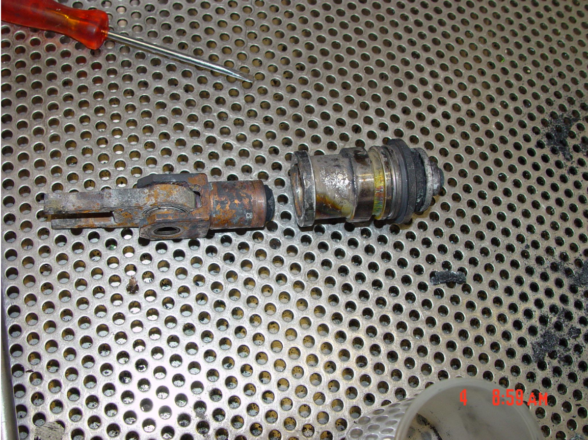
Figure 16. Driving Side Locking Cam Linkage (fractured).
