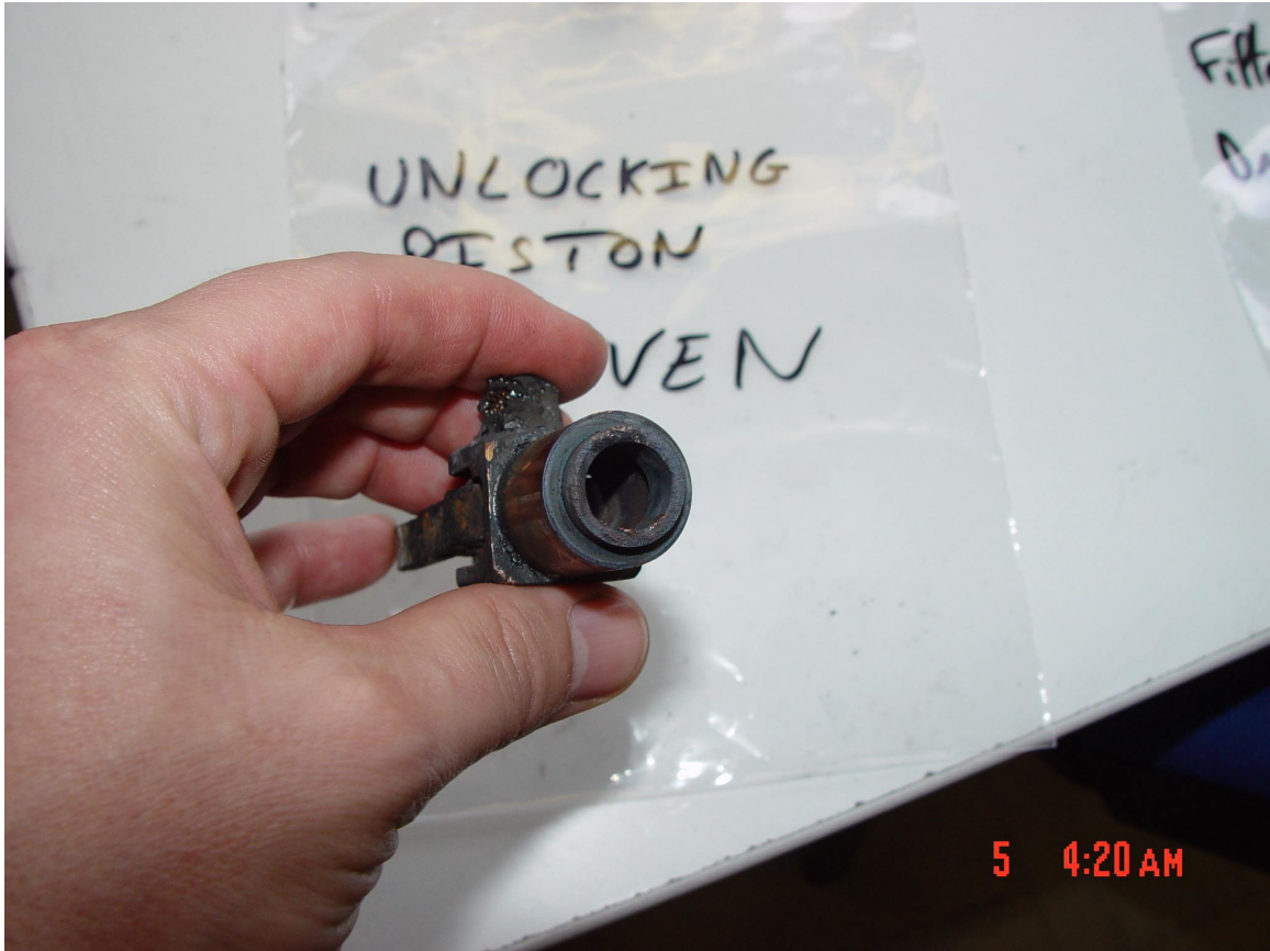
Figure 24. Driven Side Unlocking Piston and Fork (fractured).
