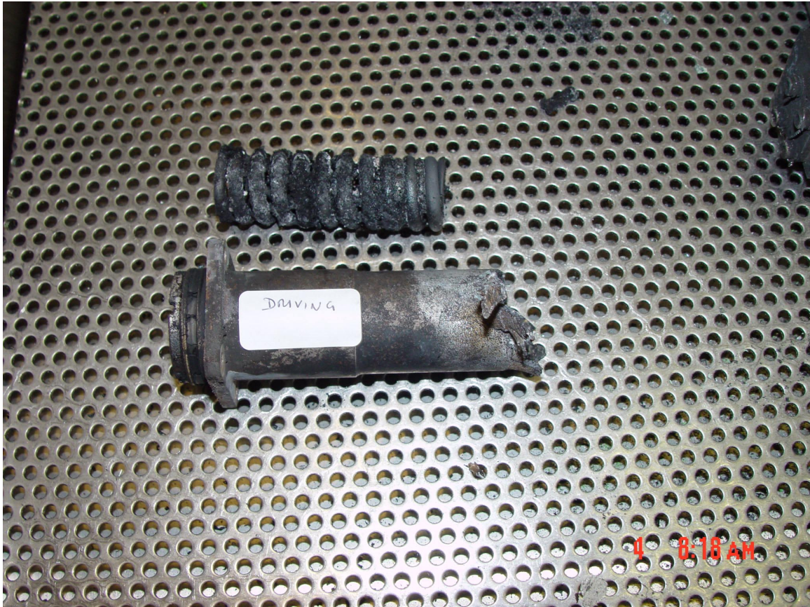
Figure 9. Driving Cylinder with Spring Removed.
