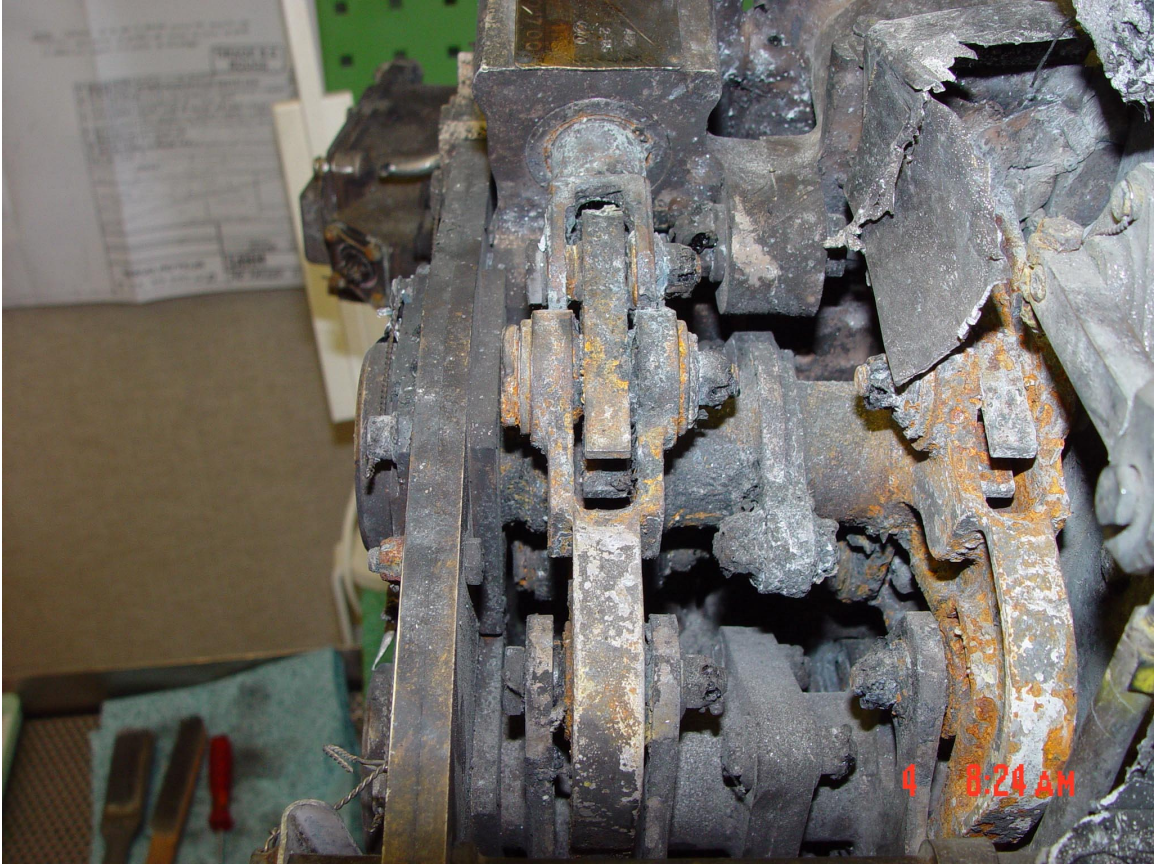
Figure 10. Driven side Locking cam linkage (left)
