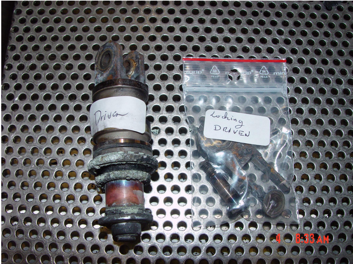
Figure 12. Driven Side Locking Linkage Removed.
