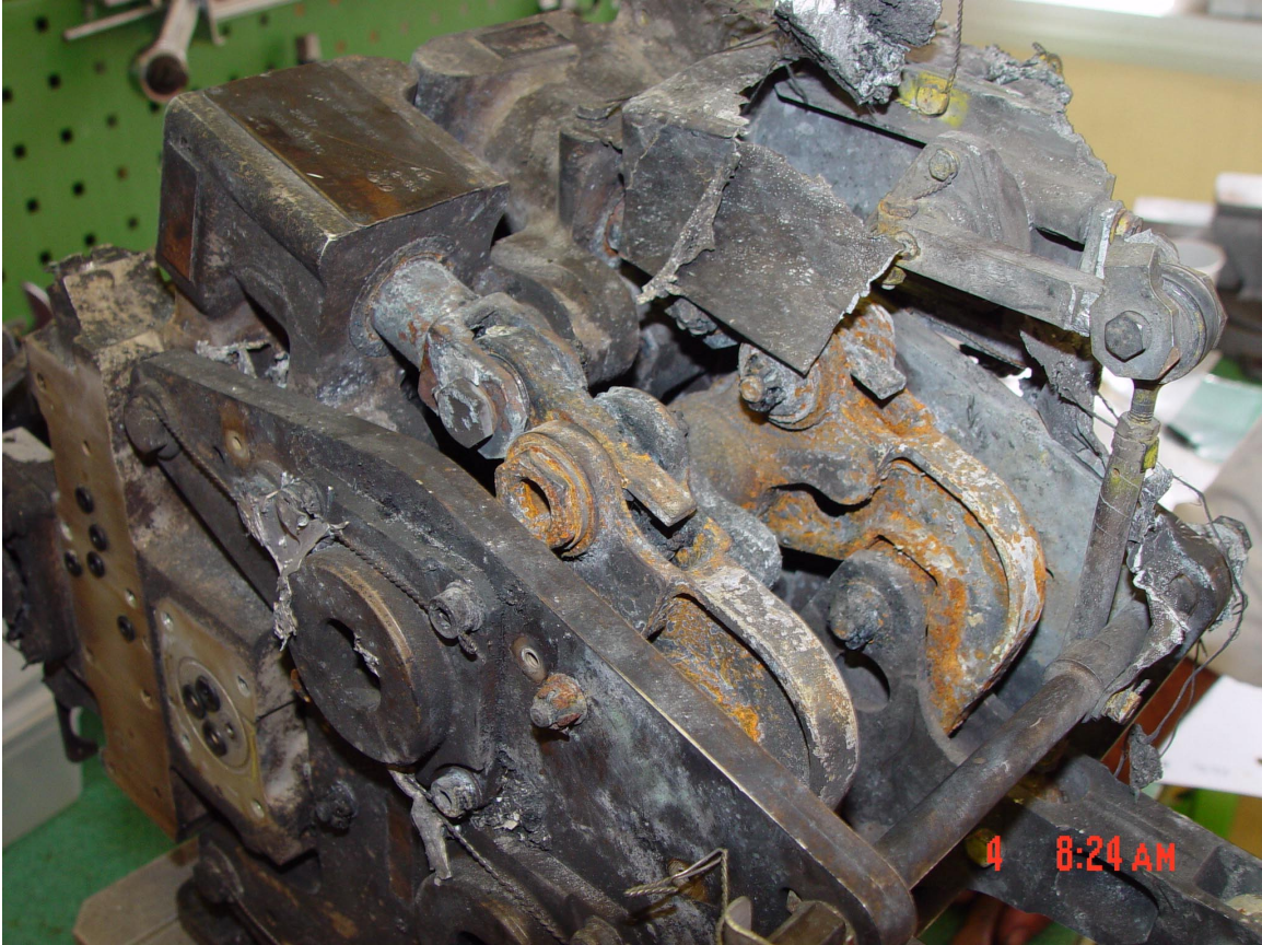
Figure 11. Driven Side Locking Cam Linkage.
