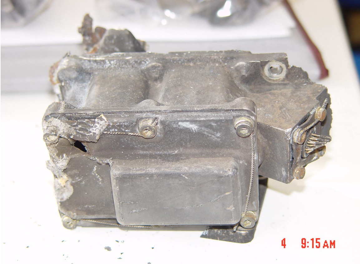
Figure 18. Driven Side Synchro Box Removed.
