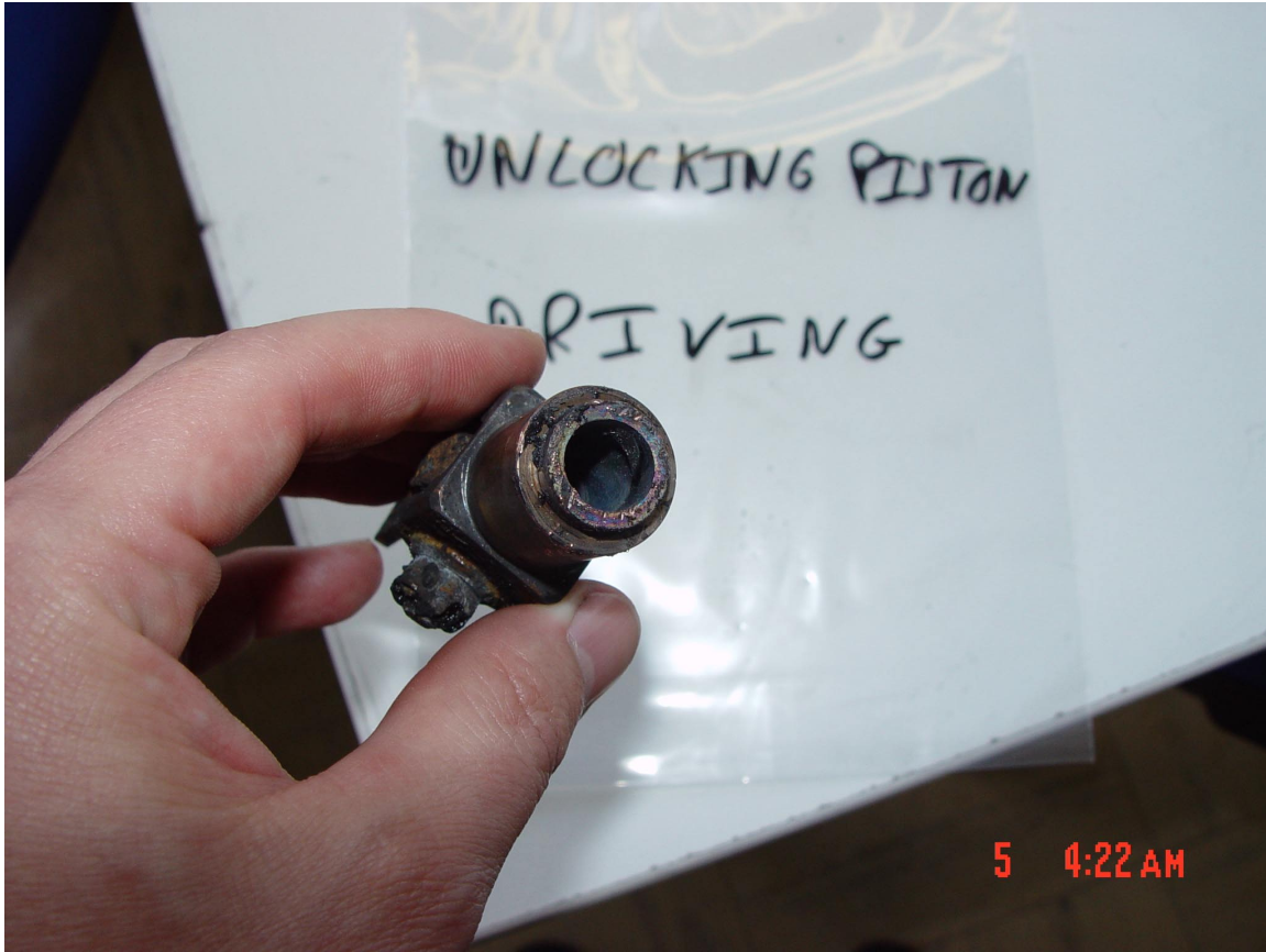
Figure 26. Driving Side Unlocking Piston and Fork (fractured).
