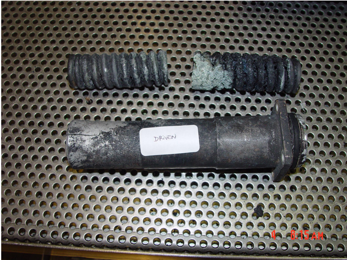
Figure 8. Driven Cylinder with Springs Removed.
