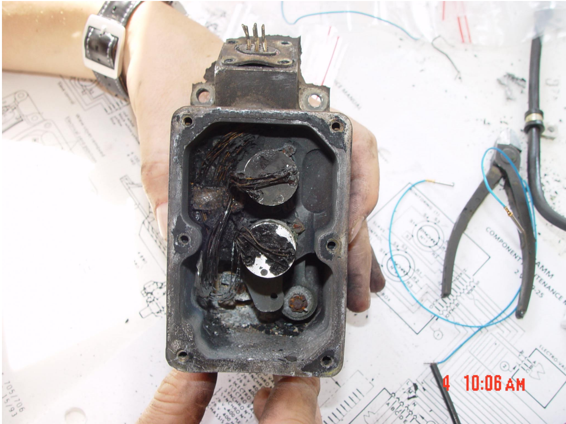
Figure 20. Driven Side Synchro Box with Cover Removed.
