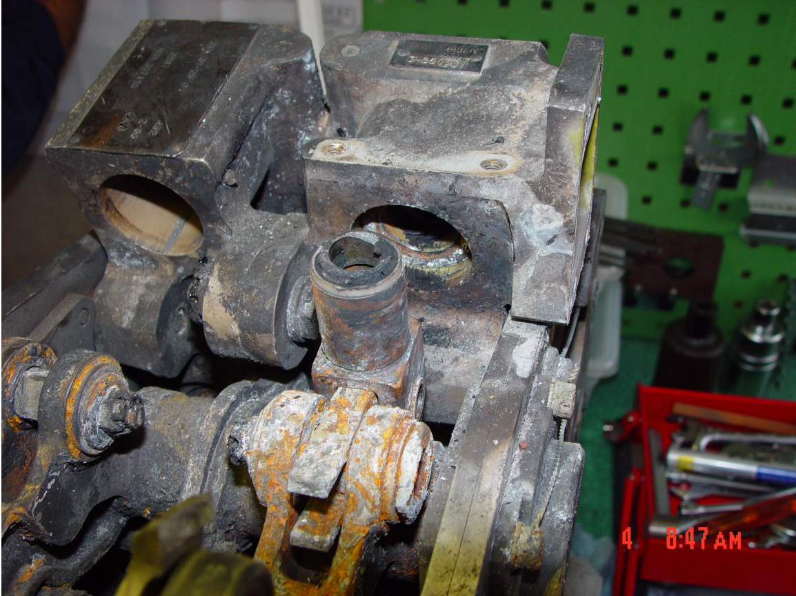
Figure 14. Driving Side Locking Cam Linkage (fractured).
