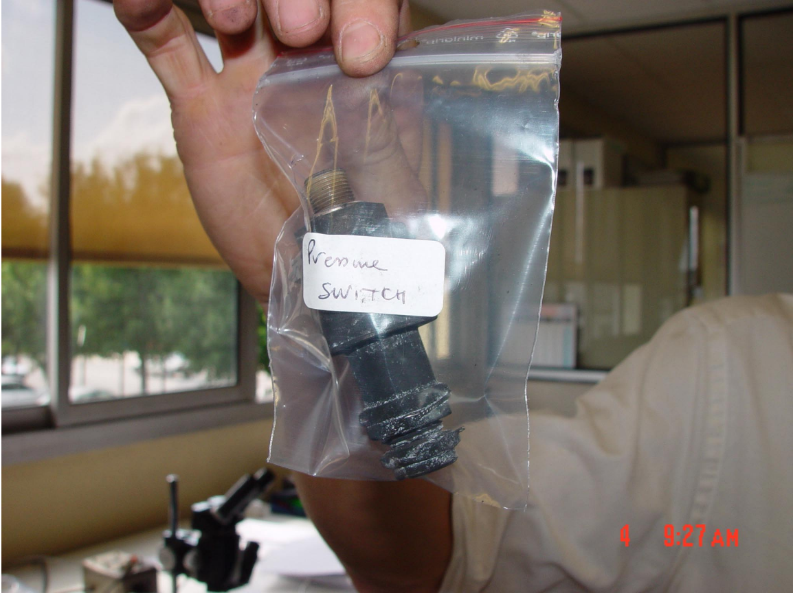
Figure 21. Engage Pressure Switch Removed.
