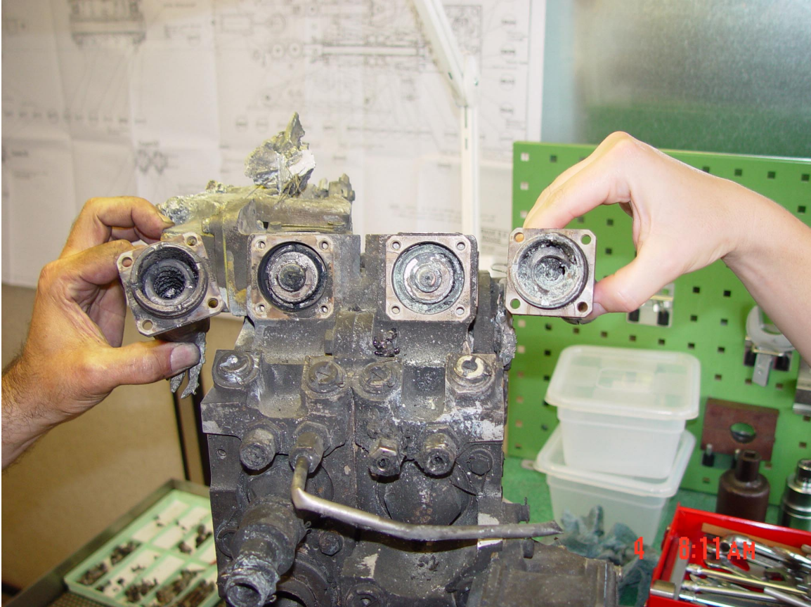
Figure 7. Driving (left) and Driven (right) Locking Cylinders Removed.
