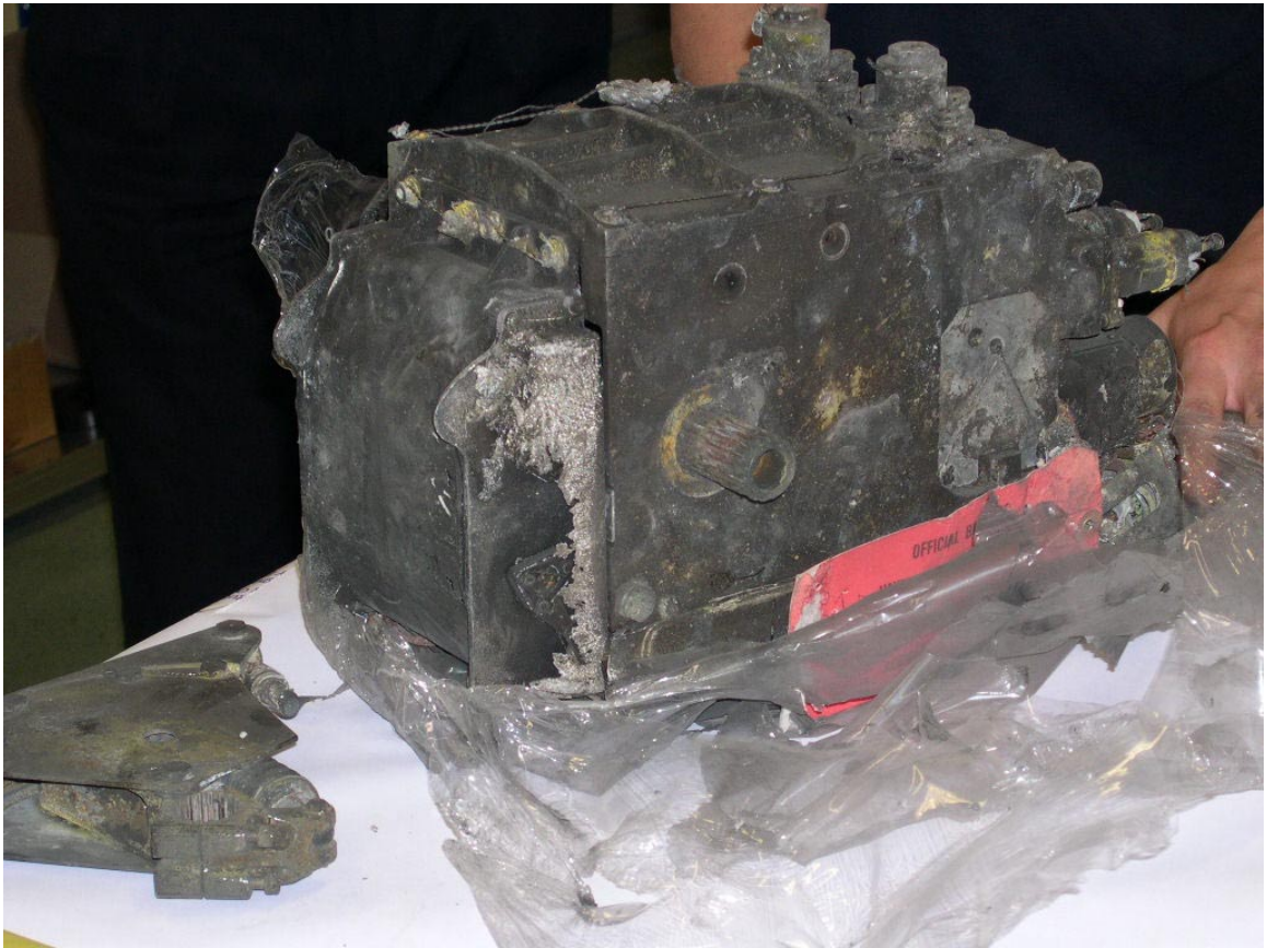
Figure 12. APSM Driving Side. Torque Limiter Removed (left, Bottom).
