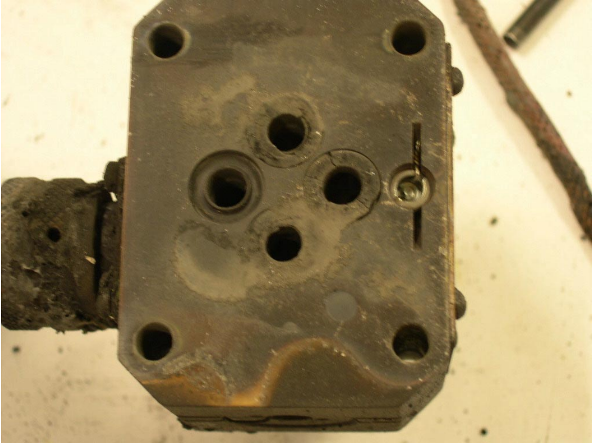
Figure 19. Driven Side Servovalve.
