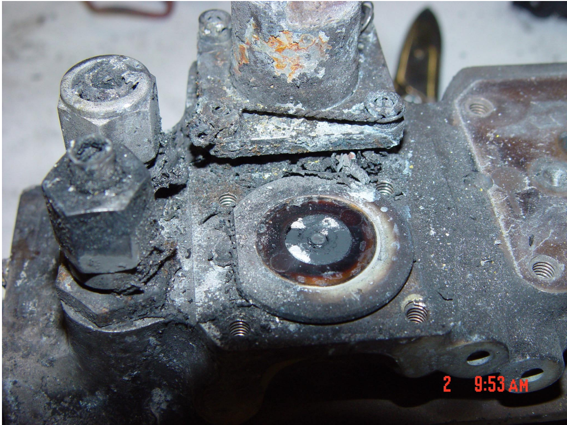
Figure 23. Driven Side With Pressure Solenoid Removed.
