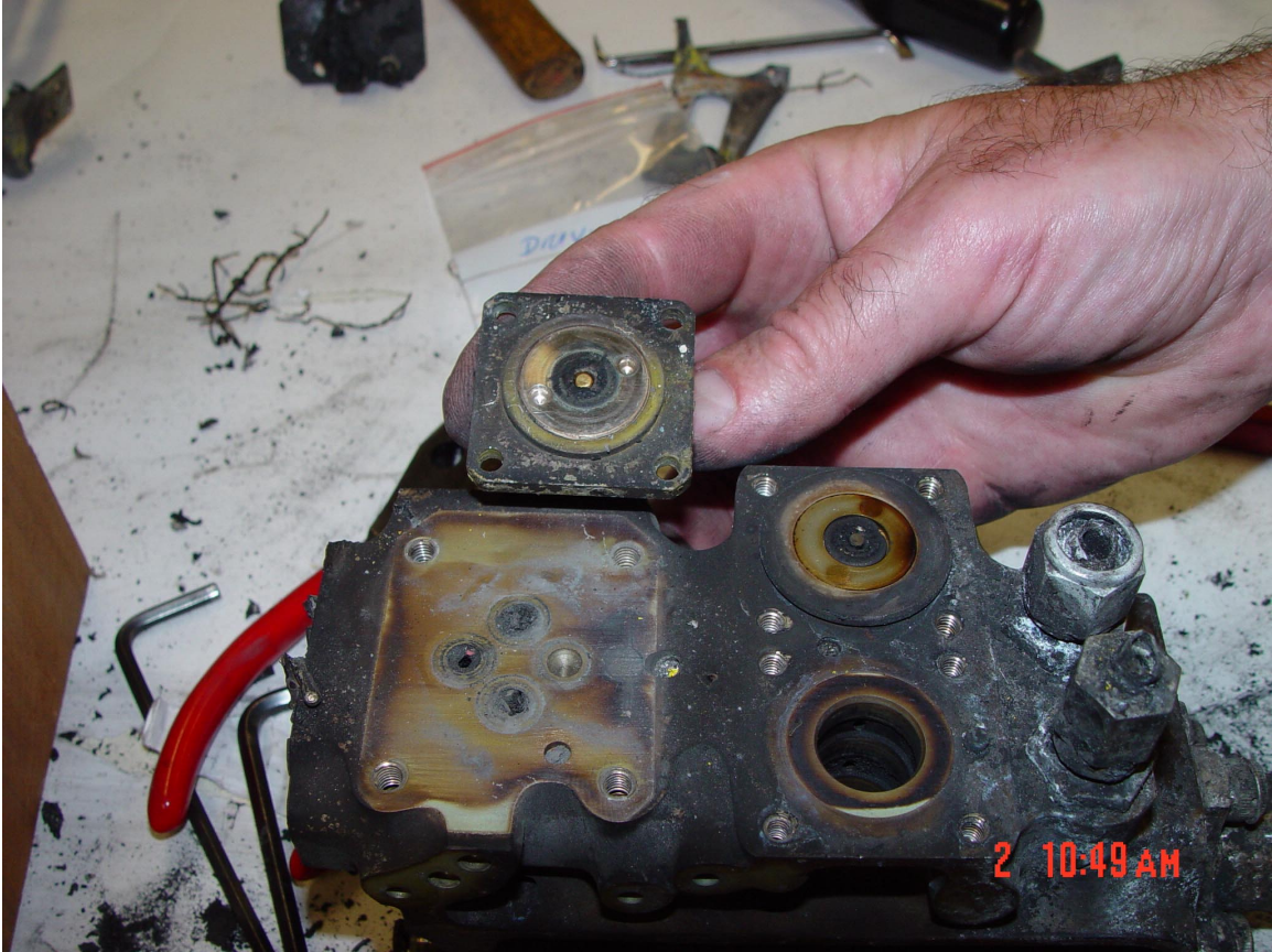
Figure 21. Driving Side With Engage Solenoid Removed.
