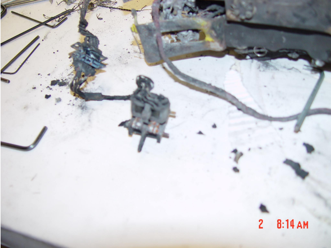
Figure 10. Driven Side Engage Switch and Wiring.
