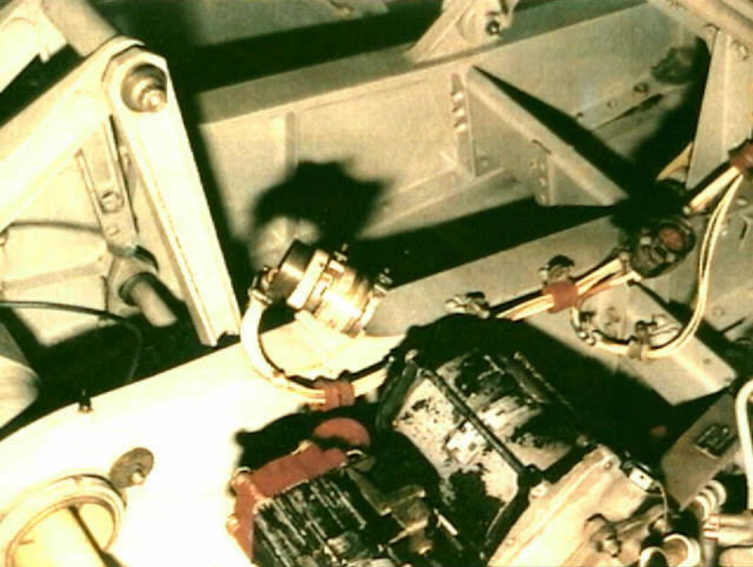
Systems 9 - 747-SL-30-048 - Fig. 29. Wire bundles to the leading edge power drive units. These bundles are susceptible to failure since these bundles are exposed to the environment during takeoff and landing. Currently-produced airpla (text cut-off).
