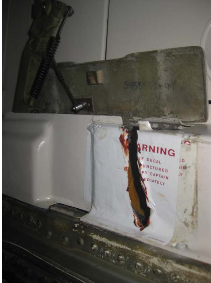
Figure 5 - Ripped tailcone placard above aft passenger door.
