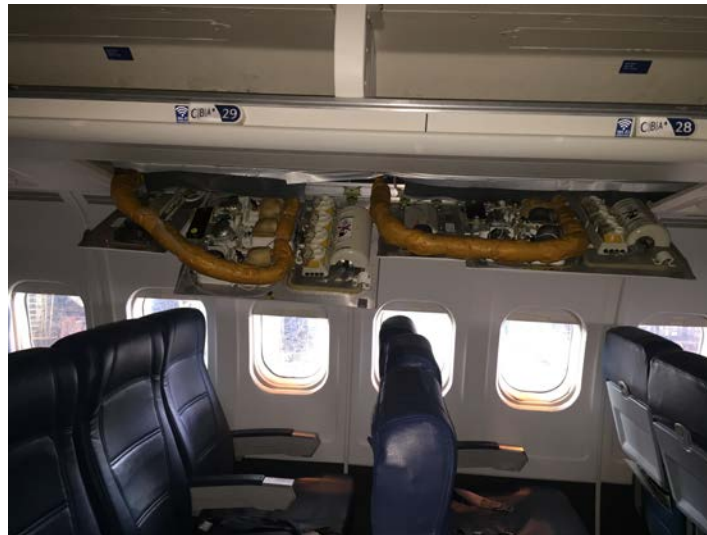
Figure 6 - Dislodged passenger service unit panels.
