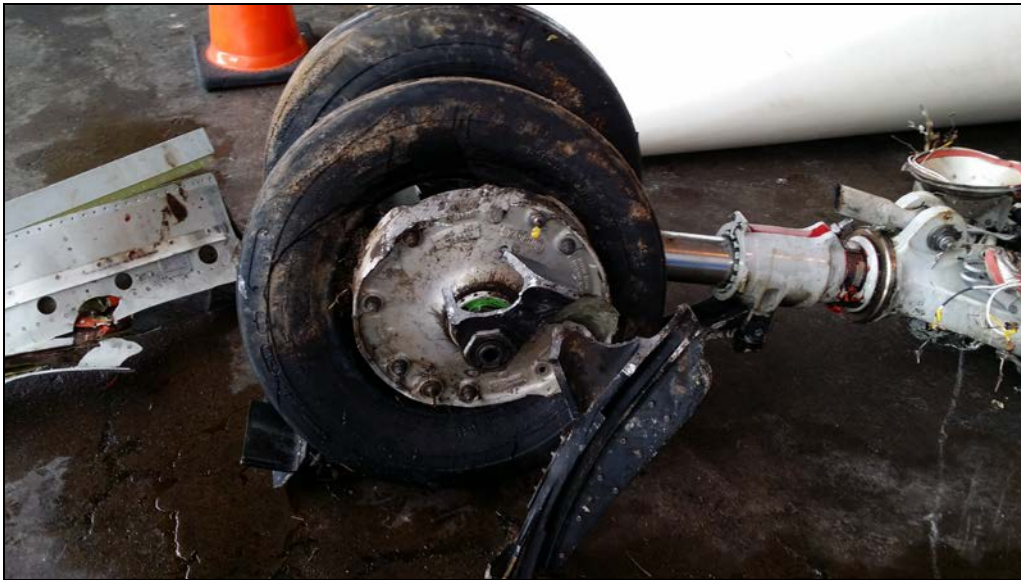
Figure 10 - Nose Landing Gear in hangar, after removal from the airplane
