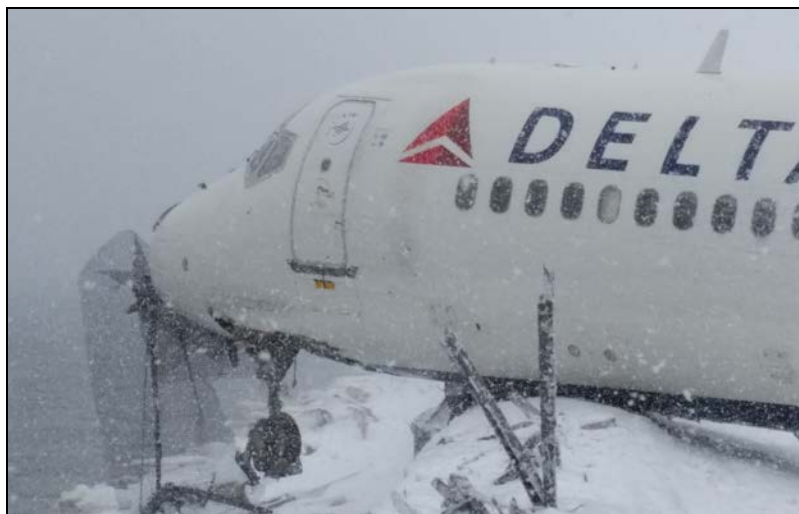
Figure 9 - Airplane on berm following the accident, prior to removal of the nose landing gear.
