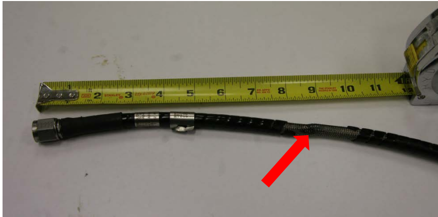
Figure 7 - Location of Hose Damage
