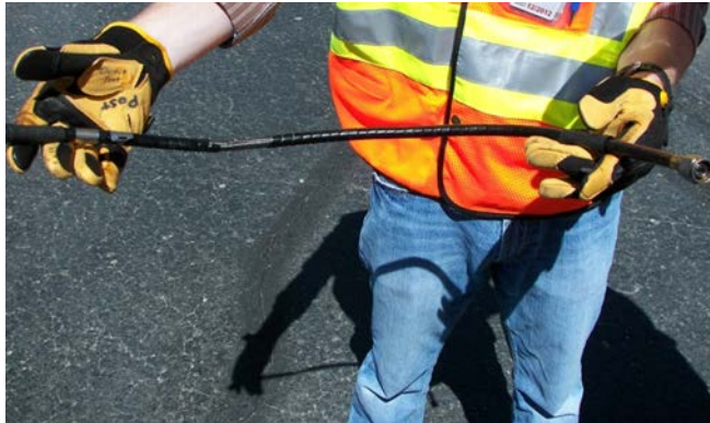
Figure 6 - The Retract Flexible Hose after removal from the airplane.
