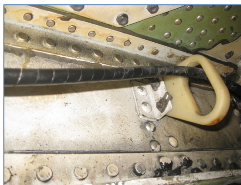
Figure 4 - Flexible Hydraulic Hose Threaded Through Guide
