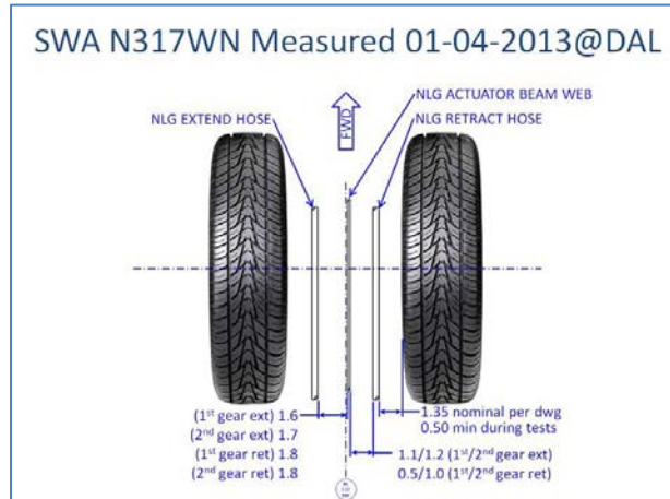
Figure 14 - Measured Clearance from Tires to Flexible Hoses
