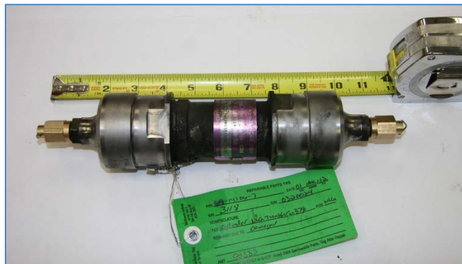
Figure 10 - Nose Landing Gear Transfer Cylinder, As Received
