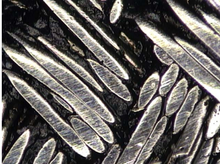
Figure 9 - Area of abrasion, magnified, showing black material located in the CRES braid.
