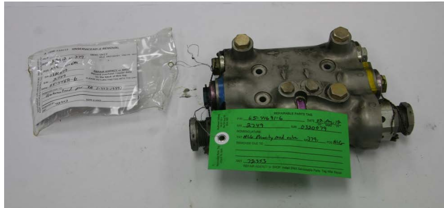
Figure 13 - Nose Landing Gear Modular Package, as Received
