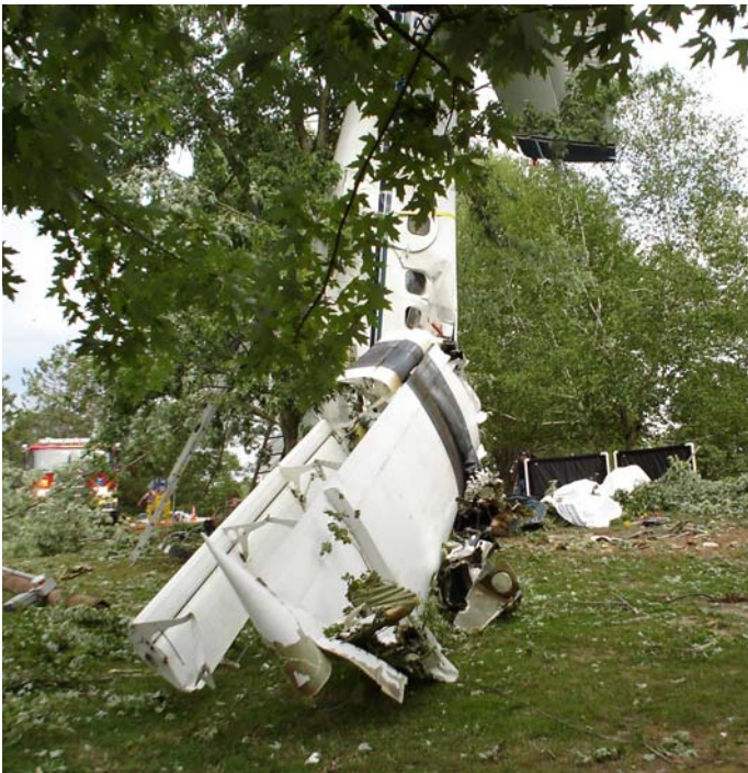
Figure 10: A photograph showing aircraft right before the right wing was removed. Wrinkling and cracking of the plane body can be seen as high as the right cabin door frame. 15
