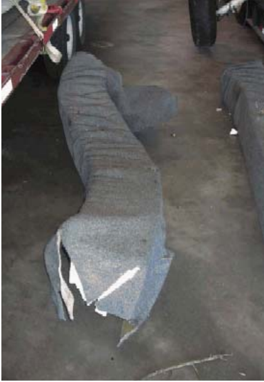
Figure 9: A post-accident photograph showing the foam cushions used for parachutist seating in the accident aircraft.
