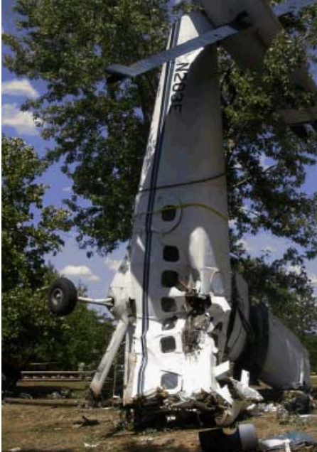
Figure 11: A photograph showing aircraft right after the right wing was removed. Crush damage can be seen immediately forward of the second window in the passenger compartment.
