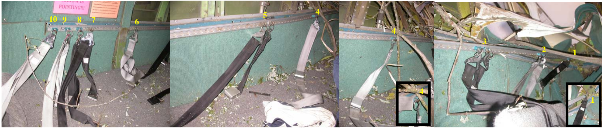
Figure 14: Post-accident photographs showing the restraints along aircraft left from back to front. The restraints are labeled as shown in Figure 13.
