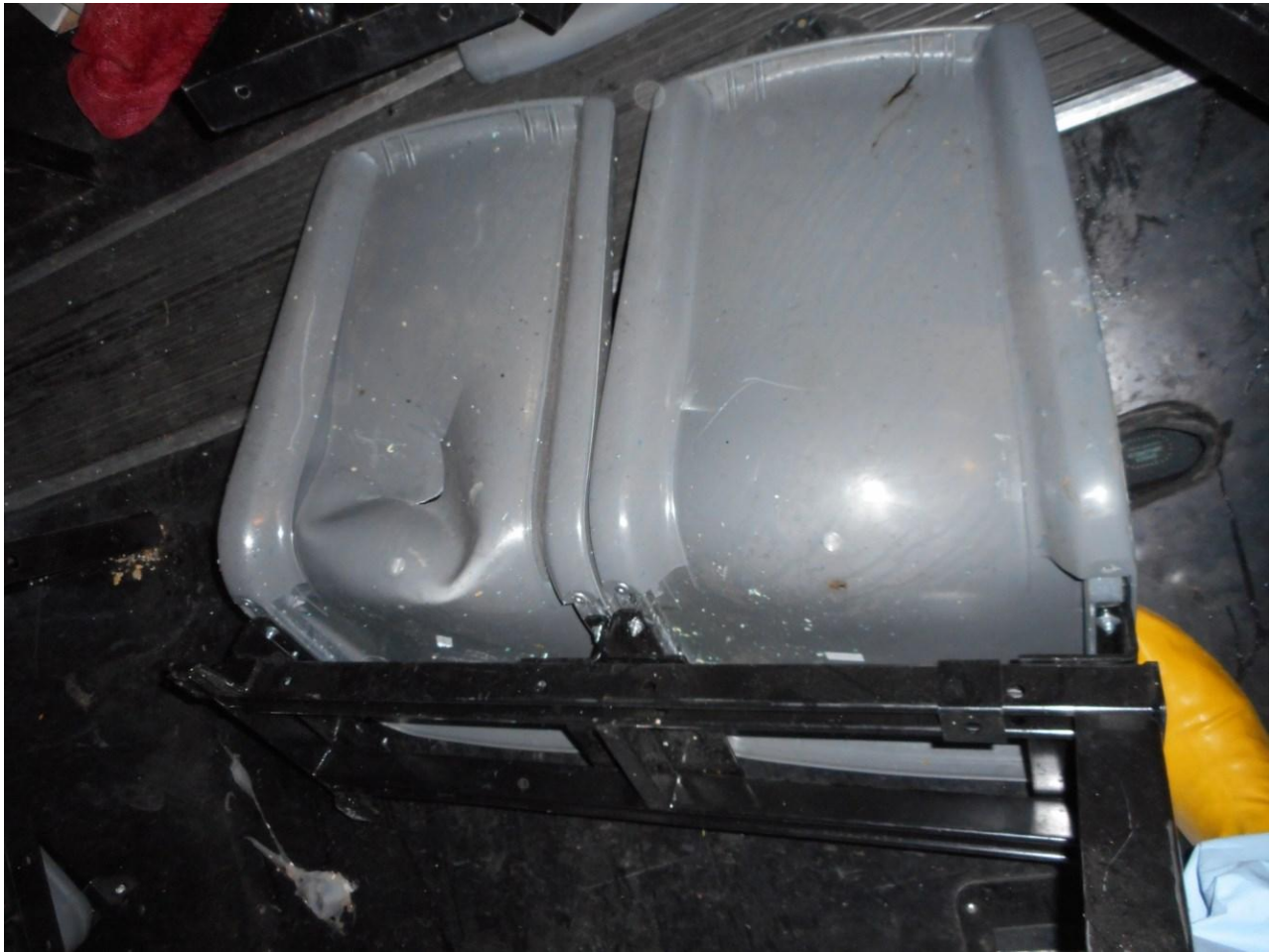
Photo 9 – View of indentation to back of seatback.
