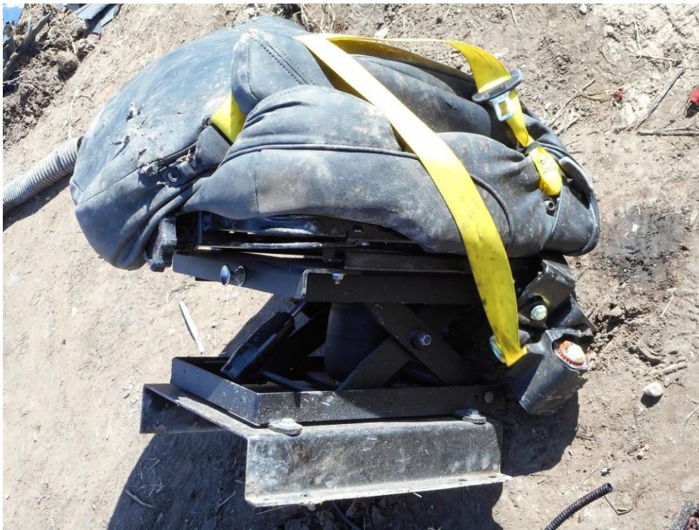
Photo 7 – View of collapsed front jump seat.
