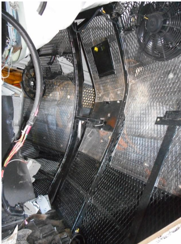
Photo 3 – View of rear caged wall showing bowing to center.
