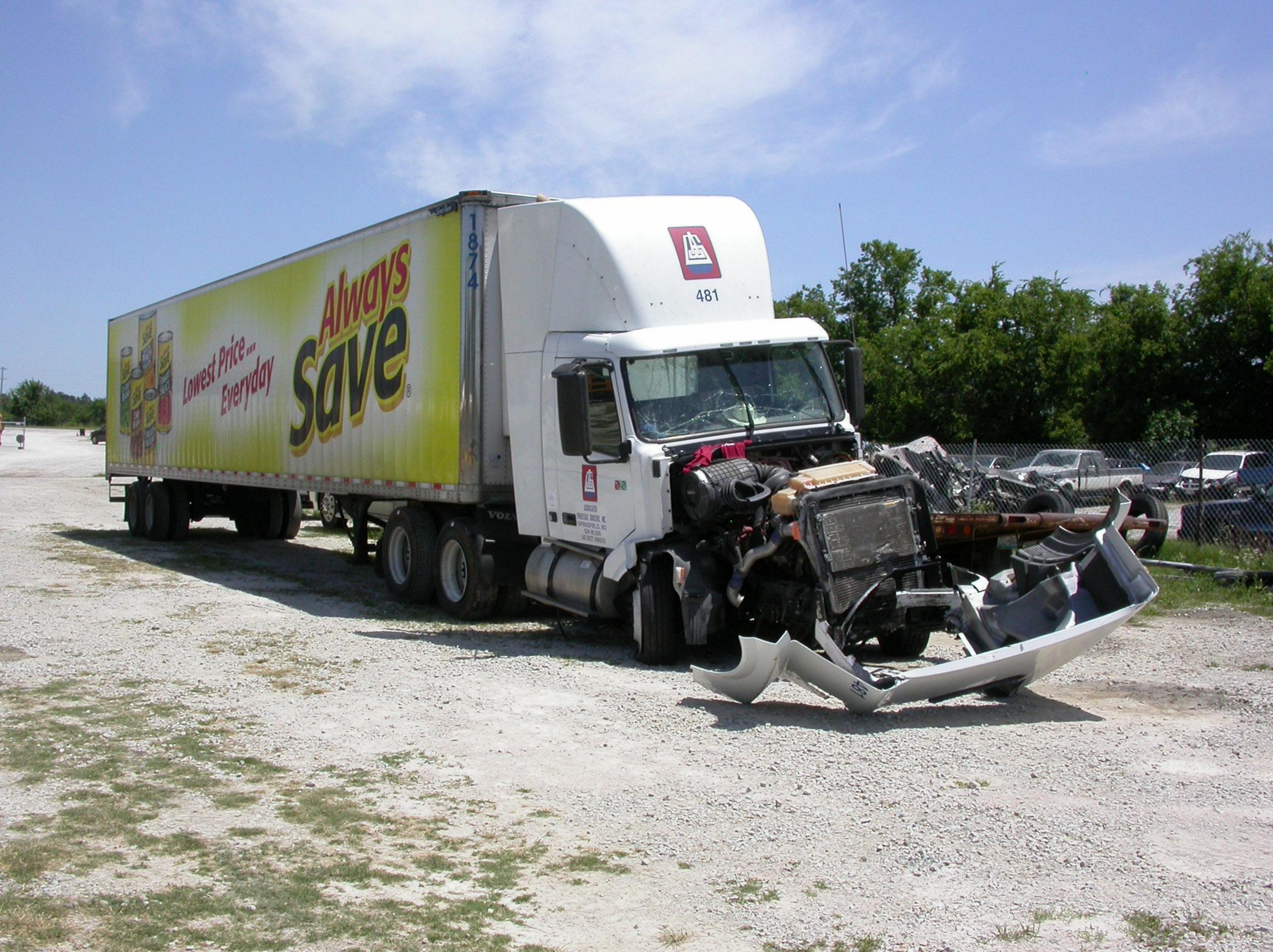
Survival Factors Photo #1 Front right angle view of damage to 2008 Volvo truck tractor
